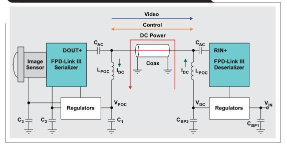
Figure 3 shows a detailed implementation of the remote camera module. An inductor,  $L_{POC}$ , is used on each side of the cable to deliver DC power. At high frequencies, the inductor presents a high impedance that blocks the AC high-speed video and low-speed control signals. The coupling capacitors,  $C_{AC}$ , block the DC power voltage so that only the AC signals are allowed to communicate between the serializer and the deserializer.
