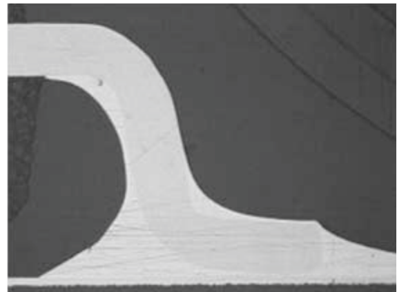
Figure 24. Cross Section of Typical NiPdAu-Finished Lead, SnAgCu Solder Paste, 255°C to 260°C Peak Reflow
