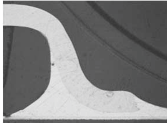
Figure 22. Cross Section of Typical Sn-Finished Lead, SnAgCu Solder Paste, 255°C to 260°C Peak Reflow
