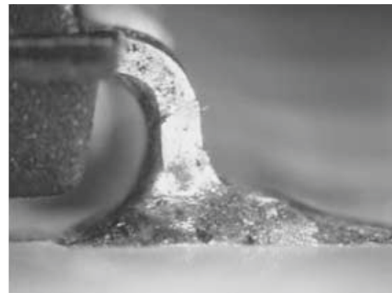
Figure 12. Typical Wetting of NiPdAu-Finished Leads With SnPbAg Solder Paste, 235°C to 240°C Peak Reflow
