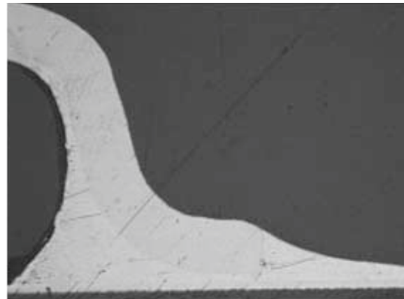
Figure 20. Cross Section of Typical NiPdAu-Finished Lead With SnPbAg Paste, 235°C to 240°C Peak Reflow
