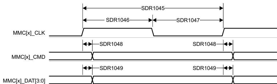
Figure 6-96. MMC1/2 – UHS-I SDR104 – Transmit Mode
