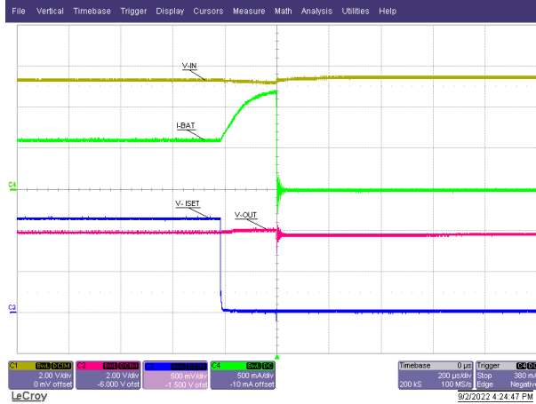
Figure 8-6. ISET Short-Circuit Response
