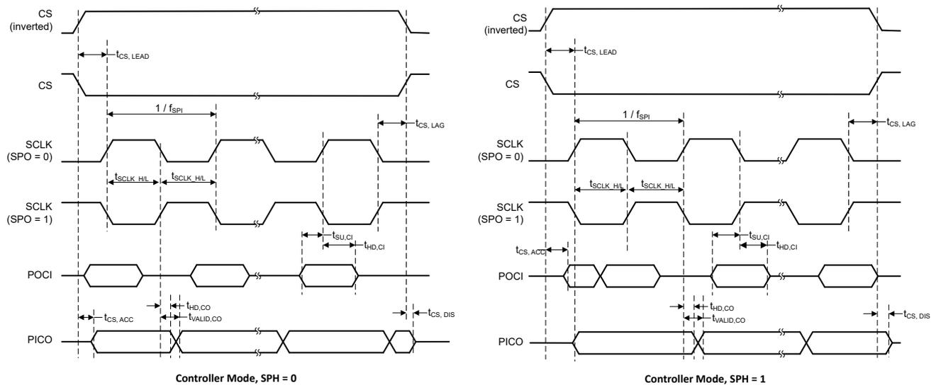
Figure 6-2. SPI Timing Diagram - Controller Mode
