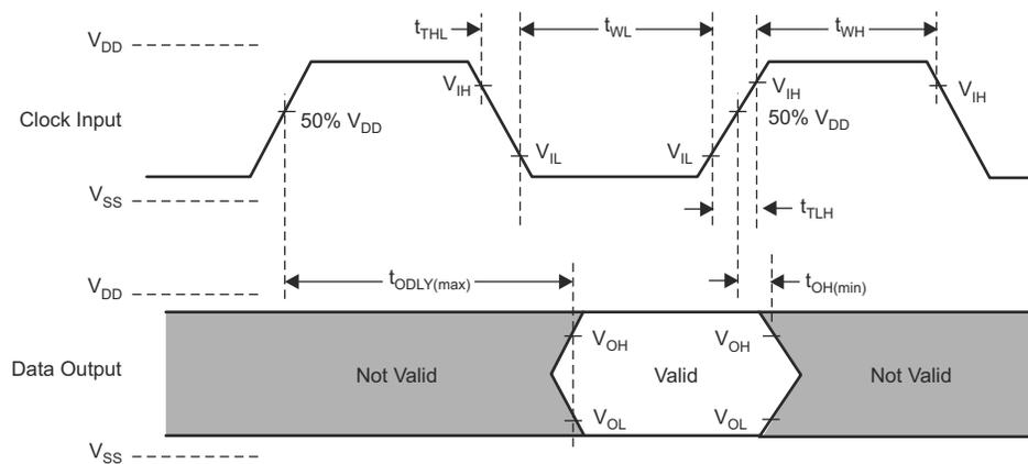
**Figure 6-7. SDIO High Speed Output Timing**
