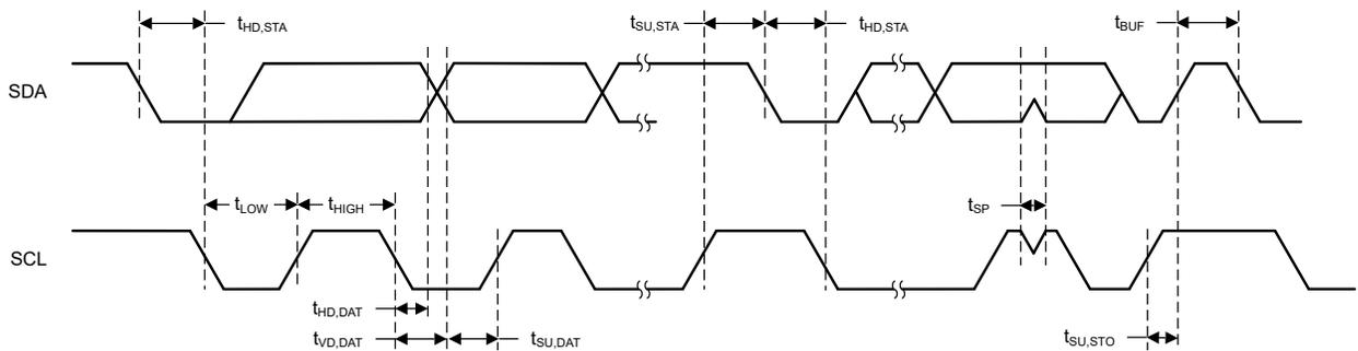
**Figure 6-1. I<sup>2</sup>C Timing Diagram**
