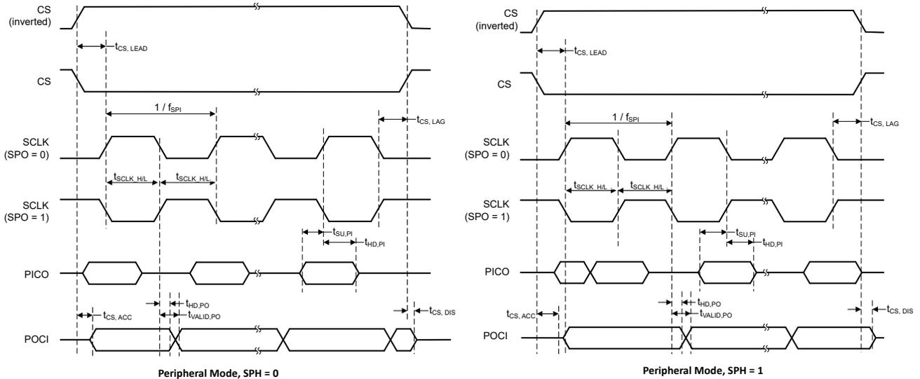
Figure 6-3. SPI Timing Diagram - Peripheral Mode
