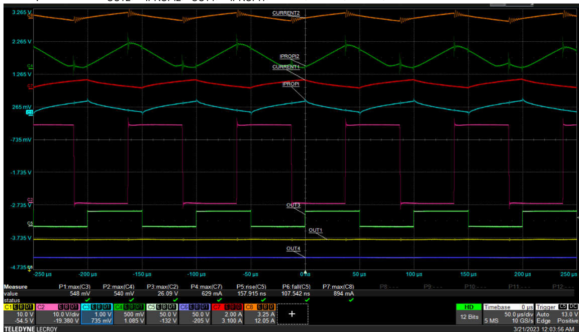
Figure 7-3. Dual H-bridge Operation, VM = 24 V
