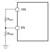
Figure 7-3. System UVLO by Enable Divider
