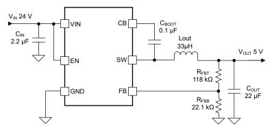
Figure 8-1. Application Circuit
