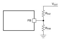
Figure 7-2. Output Voltage Setting
