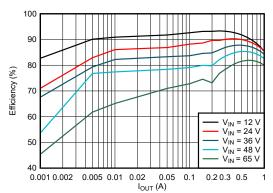
**Efficiency Versus Output Current**  $V_{OUT} = 5 \text{ V}, 400 \text{ kHz}$
