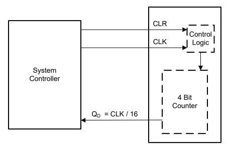
Figure 9-1. System Clock Divider
