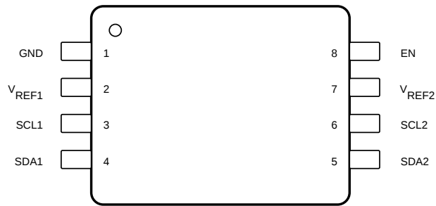
Figure 4-1. DCU Package, 8-Pin VSSOP, Top View
