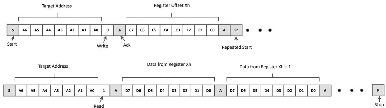
Figure 8-13. I2C Read with Repeated Start
