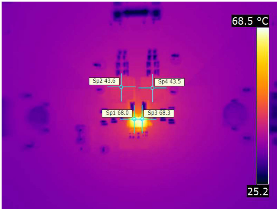
Figure 10-3. Thermal Image at 25°C Ambient - 2-phase Operation, f_{sw} = 1 MHz, V_{IN} = 12 V, V_{OUT} = 1 V, I_{OUT} = 12 A, Inductor = 560 nH (3.3 mΩ typical)
