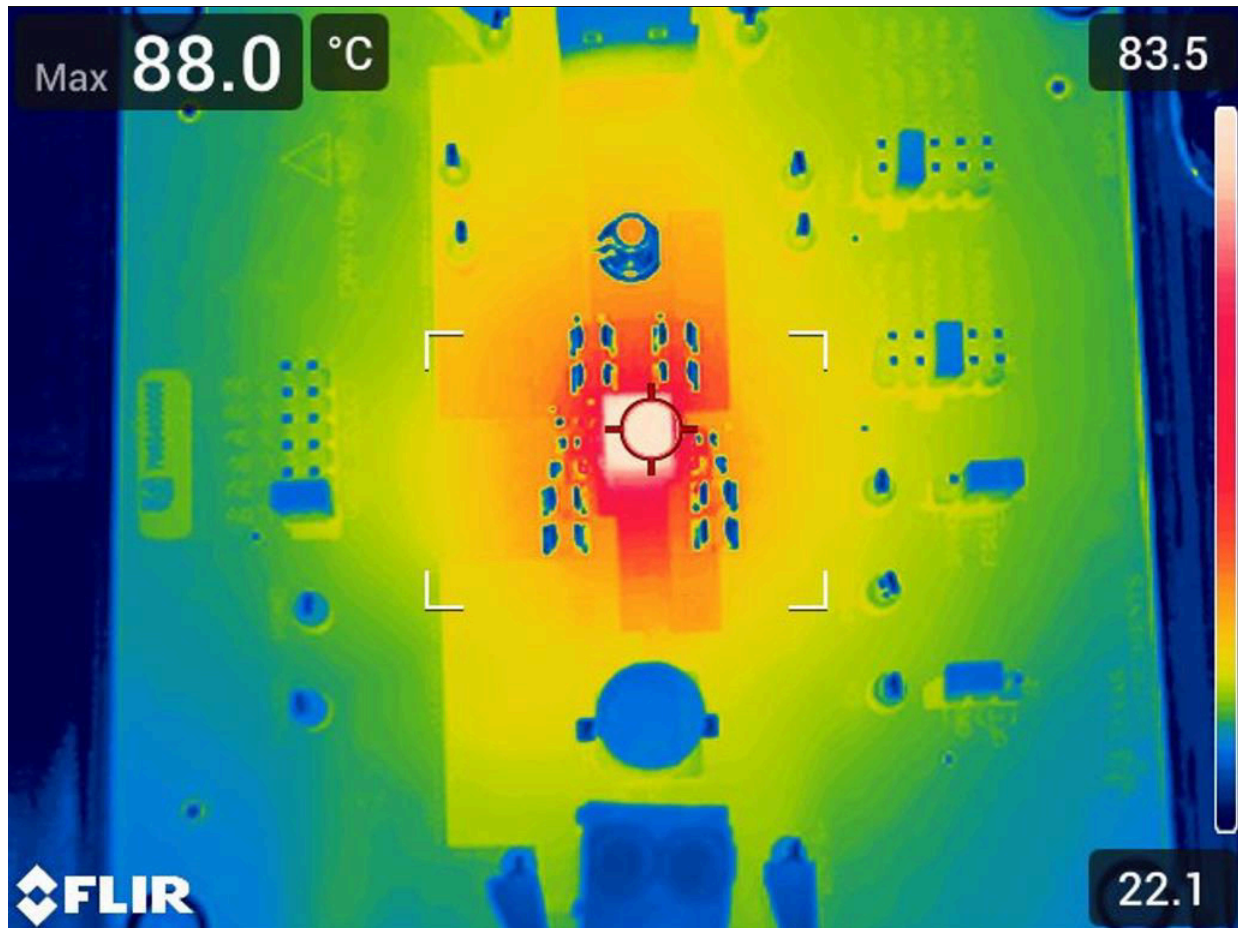
Figure 8-18. Thermal Image at 25^\circ\text{C} Ambient
