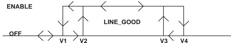
Figure 2. Line UVLO and OVLO Operation
