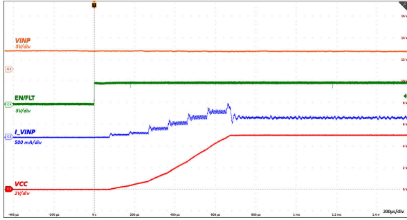
Figure 6-13. Start-Up with En/FLT From Low to High: VINP = 5.0V , VCC = 5.0V , 18Ω Load
