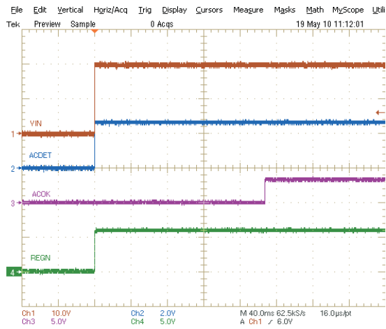
CH1: VCC, 10V/div, CH2: ACDET, 2V/div, CH3: ACOK, 5V/div, CH4: REGN, 5V/div, 40ms/div
