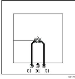
Max  $R_{\theta JA}$  = 65°C/W when mounted on 1in<sup>2</sup> (6.45cm<sup>2</sup>) of 2oz (0.071mm) thick Cu.
