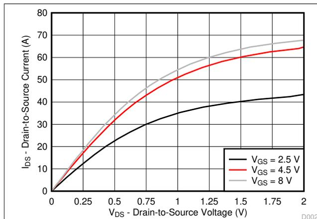
Figure 4-2. Saturation Characteristics
