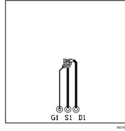
Max  $R_{\theta JA}$  = 250°C/W when mounted on a minimum pad area of 2oz (0.071mm) thick Cu.
