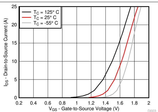
Figure 4-3. Transfer Characteristics
