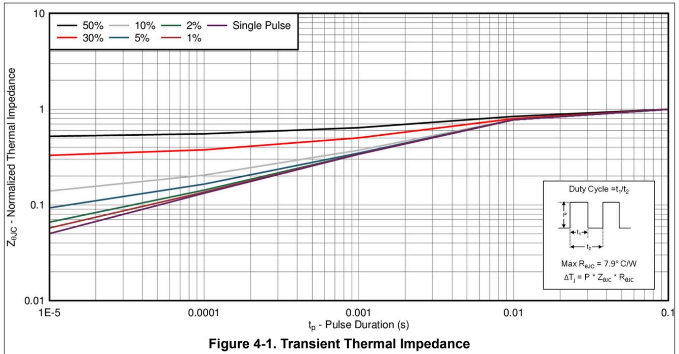
Figure 4-1. Transient Thermal Impedance
