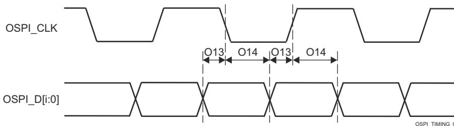
**Figure 6-117. OSPI Timing Requirements – Tap DDR, No Loopback**
