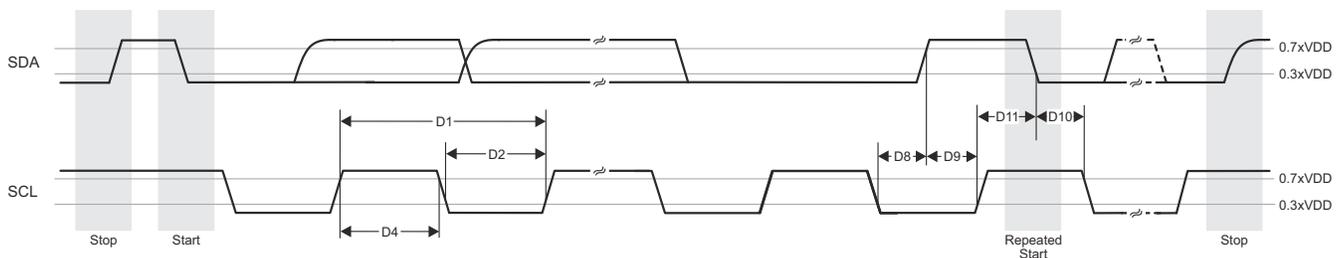
**Figure 6-83. I3C Push-Pull Timing Requirements - SDR Mode**
