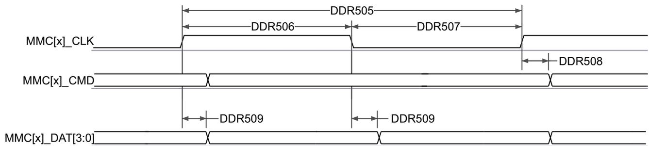
**Figure 6-106. MMC1/2 – UHS-I DDR50 – Transmit Mode**
