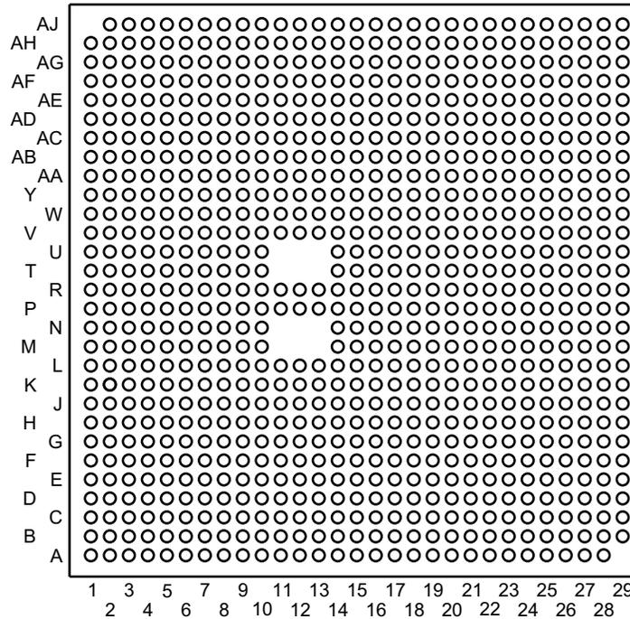
**Figure 5-1. ALF FCBGA-N827 Pin Diagram (Bottom View)**
