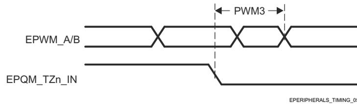
**Figure 6-60. EPWM\_A/B and ePWM\_TZn\_IN Forced High/Low Input Timings**
