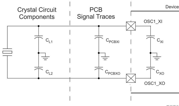
**Figure 6-30. Load Capacitance**
