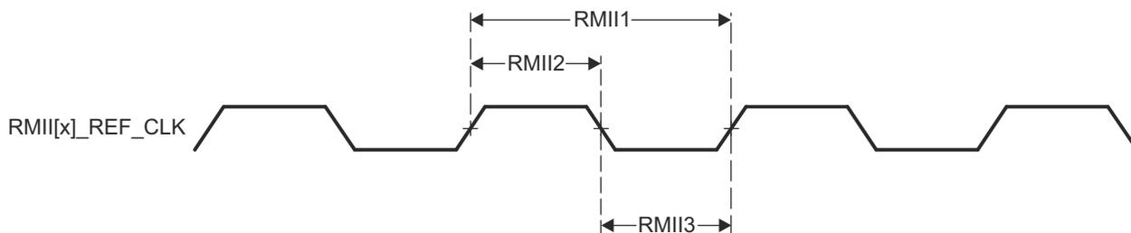
**Figure 6-48. RMII[x]\_REF\_CLK Timing Requirements – RMII Mode**
