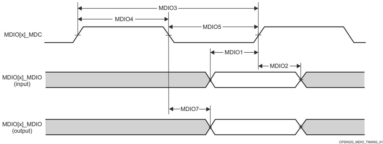
**Figure 6-47. CPSW9G MDIO Diagrams Receive and Transmit**
