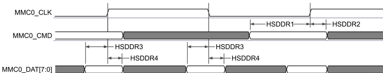
**Figure 6-94. MMC0 – High Speed DDR Mode – Receive Mode**
