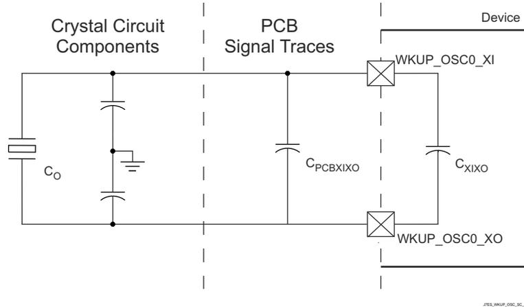
Figure 6-26. Shunt Capacitance
