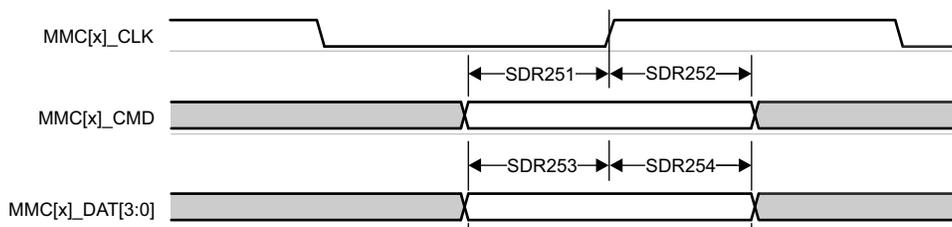
**Figure 6-103. MMC1/2 – UHS-I SDR25 – Receive Mode**
