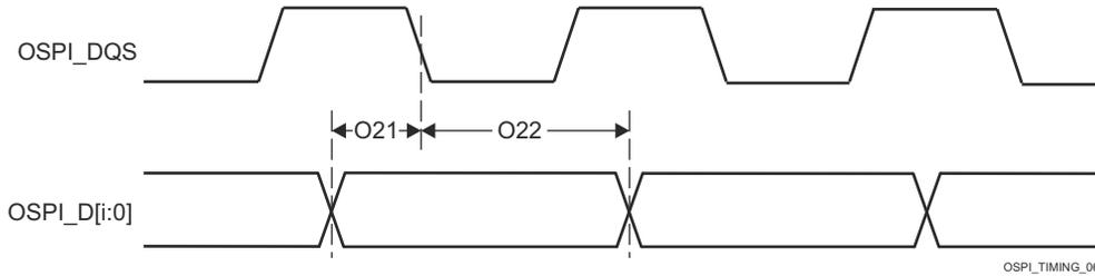
**Figure 6-111. OSPI Timing Requirements – SDR, External Loopback Clock**
