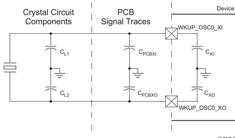
**Figure 6-25. Load Capacitance**
