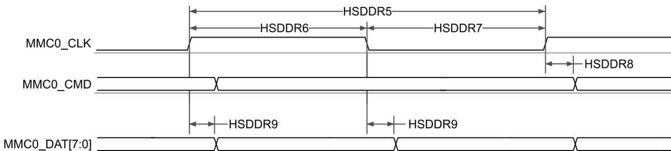
**Figure 6-95. MMC0 – High Speed DDR Mode – Transmit Mode**
