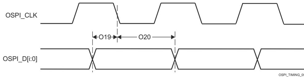
**Figure 6-115. OSPI Timing Requirements – Tap SDR, No Loopback**
