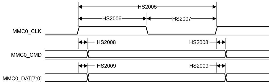
**Figure 6-96. MMC0 – HS200 Mode – Transmit Mode**
