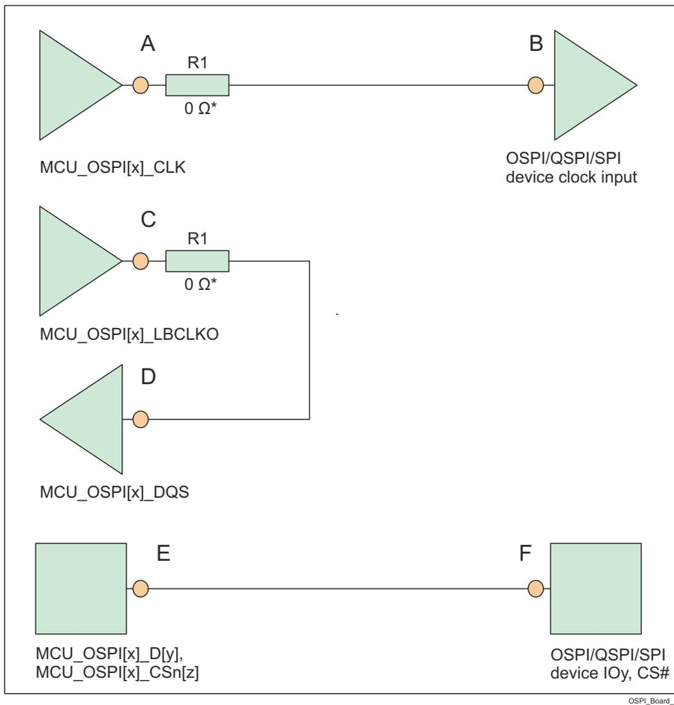
\* 0 Ω resistor (R1), located as close as possible to the MCU\_OSPI[x]\_CLK and MCU\_OSPI[x]\_LBCLKO pins, is a placeholder for fine tuning, if needed.
