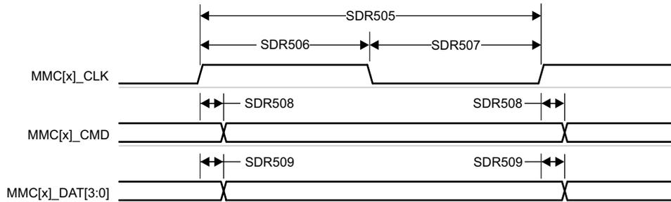
**Figure 6-105. MMC1/2 – UHS-I SDR50 – Transmit Mode**
