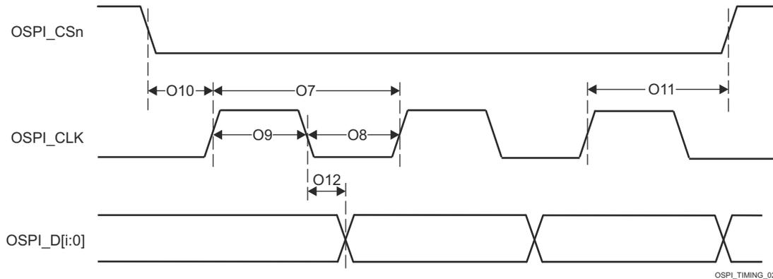
**Figure 6-116. OSPI Switching Characteristics – Tap SDR, No Loopback**
