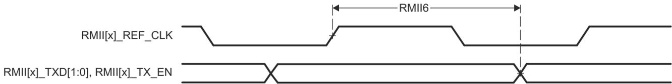
Figure 6-50. RMII[x]\_TXD[1:0], and RMII[x]\_TX\_EN Switching Characteristics – RMII Mode
