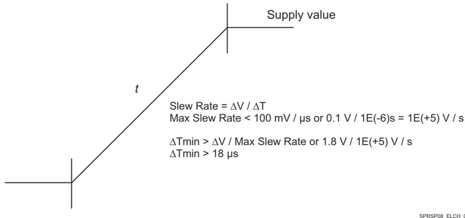
**Figure 6-2. Power Supply Slew and Slew Rate**
