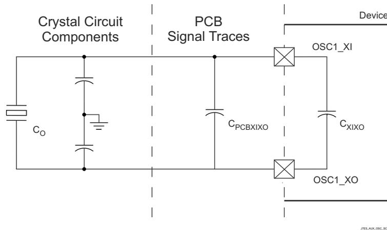
**Figure 6-31. Shunt Capacitance**
