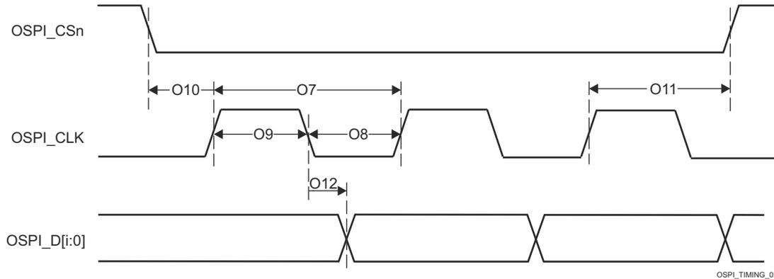
**Figure 6-112. OSPI Switching Characteristics – SDR**
