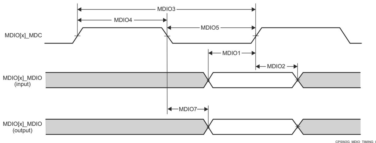
**Figure 6-41. CPSW2G MDIO Timing Requirements and Switching Characteristics**
