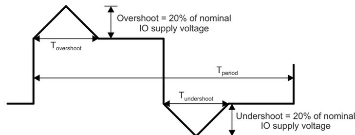
A.  $T_{\text{overshoot}} + T_{\text{undershoot}} < 20\% \text{ of } T_{\text{period}}$
