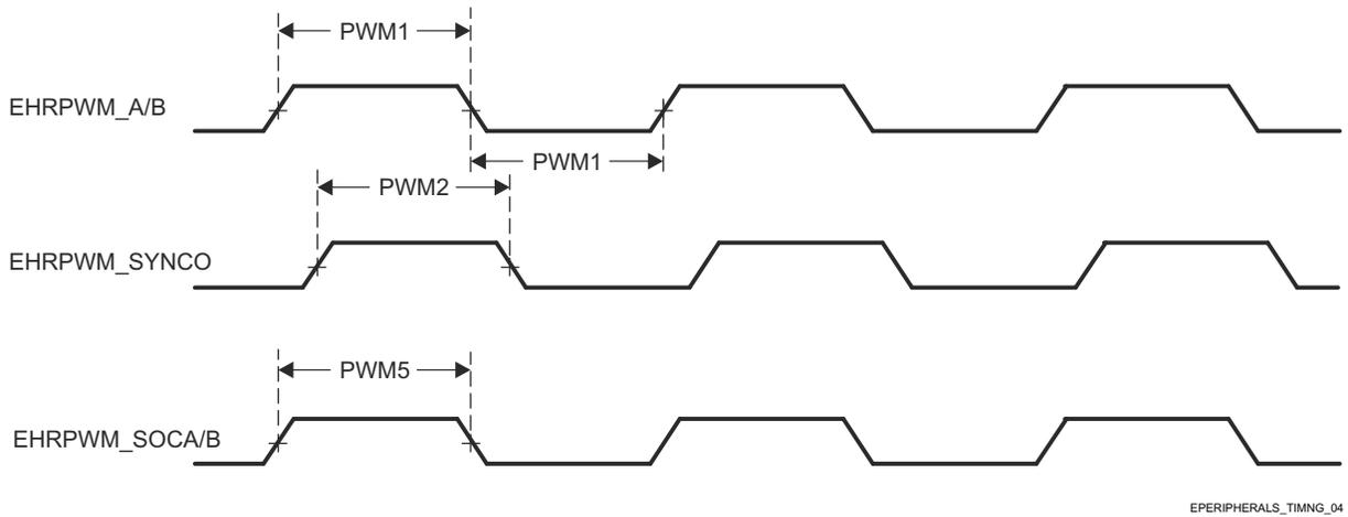
**Figure 6-59. EPWM\_A/B\_out, ePWM\_SYNCO, and ePWM\_SOC A/B Input Timings**
