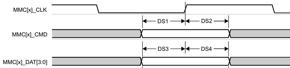
**Figure 6-97. MMC1/2 – Default Speed – Receive Mode**
