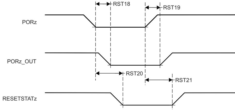
**Figure 6-12. PORz initiates; PORz\_OUT and RESETSTATz Switching Characteristics**
