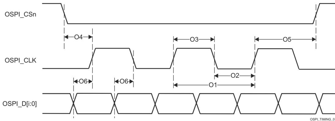
**Figure 6-118. OSPI Switching Characteristics – Tap DDR, No Loopback**
