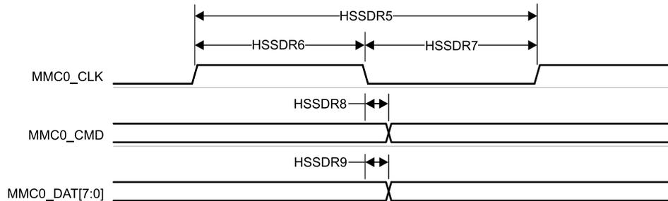
**Figure 6-93. MMC0 – High Speed SDR Mode – Transmit Mode**
