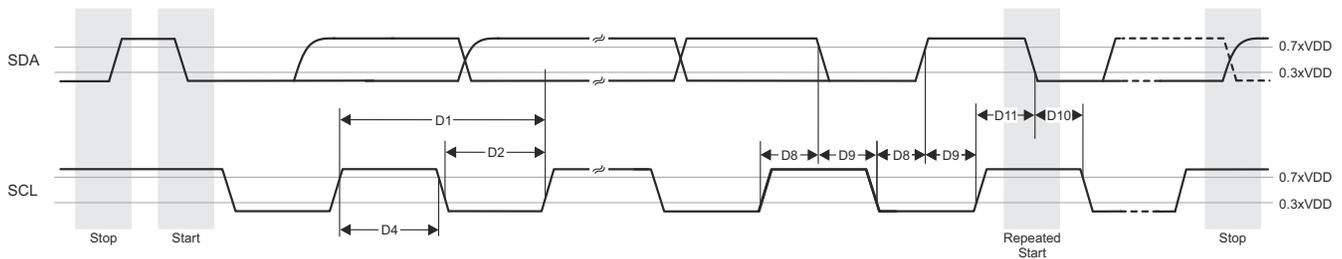
**Figure 6-82. I3C Push-Pull Timing Requirements - HDR-DDR Mode**
