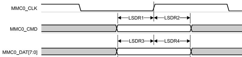
**Figure 6-90. MMC0 – Legacy SDR – Receive Mode**
