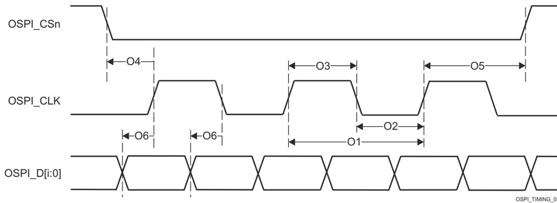
**Figure 6-114. OSPI Switching Characteristics – DDR**
