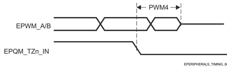
**Figure 6-61. EPWM\_A/B and ePWM\_TZn\_IN Hi-Z Input Timings**
