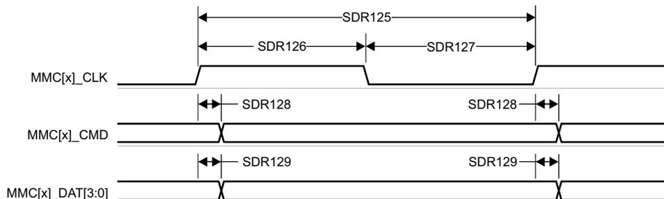
Figure 6-102. MMC1/2 – UHS-I SDR12 – Transmit Mode
