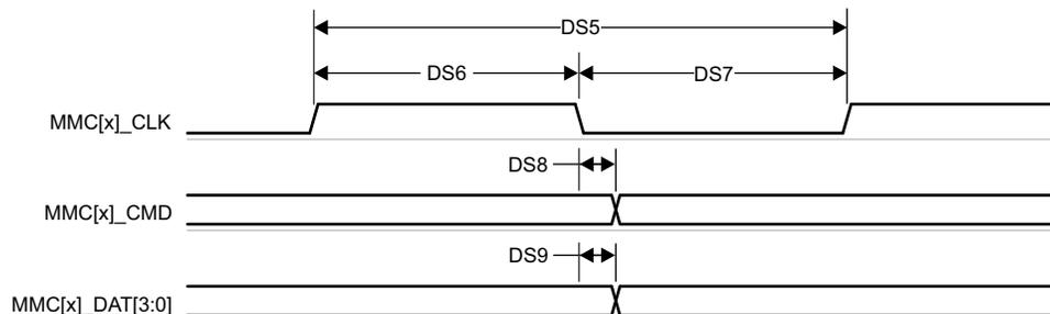
**Figure 6-98. MMC1/2 – Default Speed – Transmit Mode**
