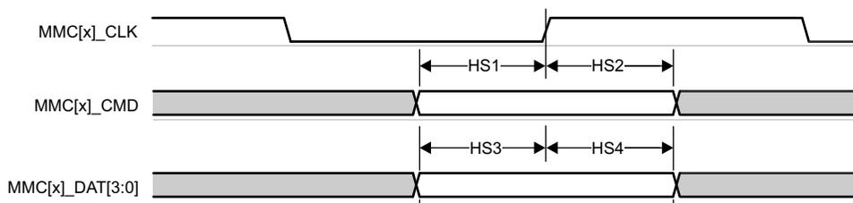
**Figure 6-99. MMC1 /2– High Speed – Receive Mode**
