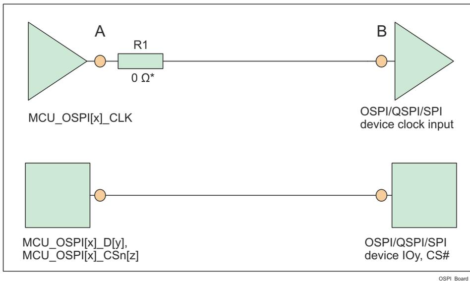
\*  $0\ \Omega$  resistor (R1), located as close as possible to the MCU\_OSPI[x]\_CLK pin, is placeholder for fine tuning, if needed.
