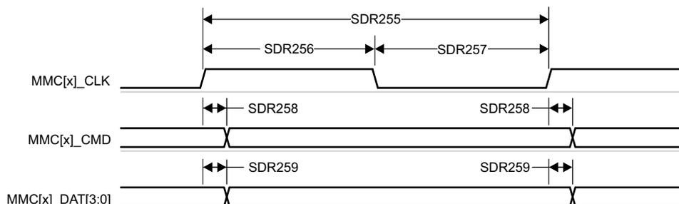
**Figure 6-104. MMC1/2 – UHS-I SDR25 – Transmit Mode**
