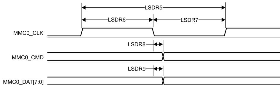
**Figure 6-91. MMC0 – Legacy SDR – Transmit Mode**
