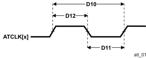
Figure 6-38. ATCLK[x] Timing
