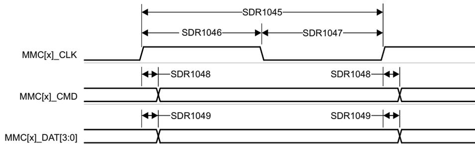
**Figure 6-107. MMC1/2 – UHS-I SDR104 – Transmit Mode**
