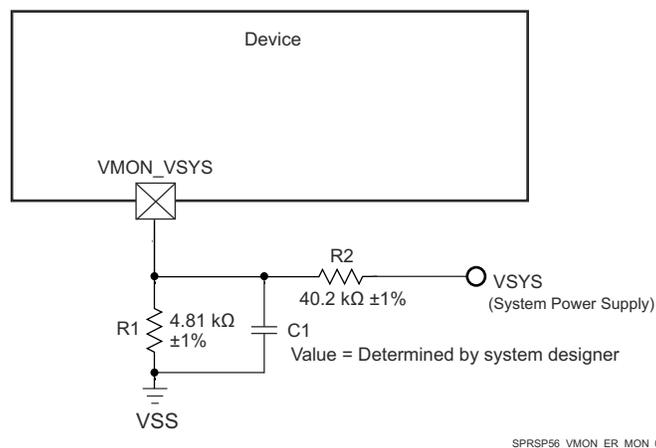
**Figure 8-5. System Supply Monitor Voltage Divider Circuit**
