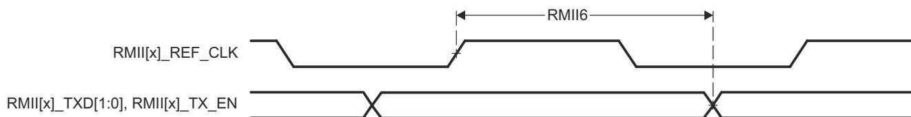
**Figure 6-44. RMII[x]\_TXD[1:0], and RMII[x]\_TX\_EN Switching Characteristics – RMII Mode**
