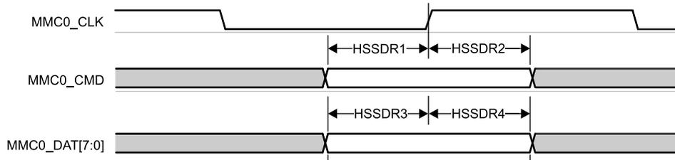
**Figure 6-92. MMC0 – High Speed SDR Mode – Receive Mode**
