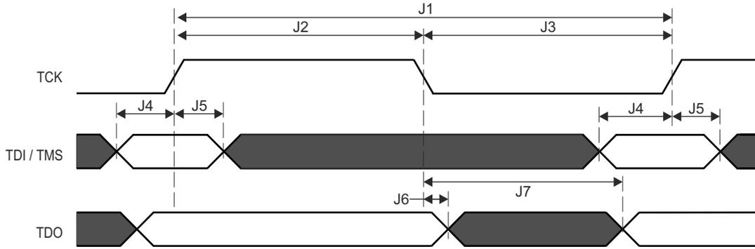
**Figure 6-122. JTAG Timing Requirements and Switching Characteristics**
