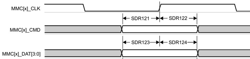
Figure 6-101. MMC1/2 – UHS-I SDR12 – Receive Mode
