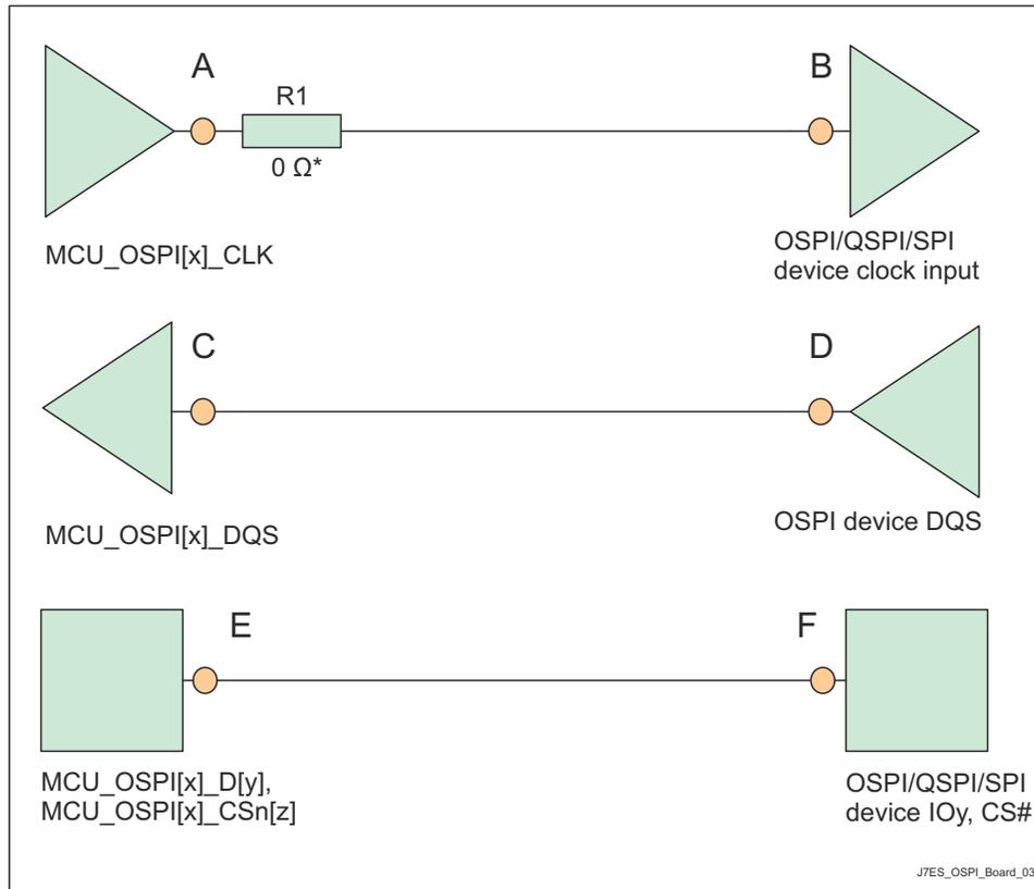
\* 0 Ω resistor (R1), located as close as possible to the MCU\_OSPI[x]\_CLK pin, is a placeholder for fine tuning, if needed.
