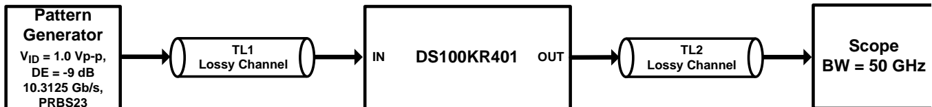
Figure 13. Test Setup Connections Diagram
