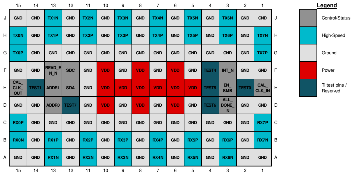
Figure 4-1. 135-Pin fcBGA, 0.8mm BGA Pin Pitch (Top View)
