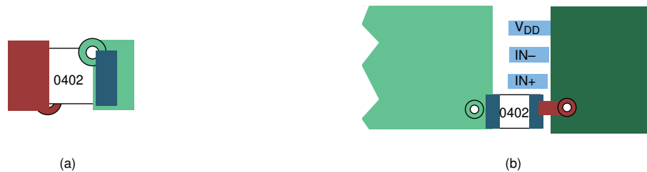
Figure 11-7. Typical Decoupling Capacitor Layouts
