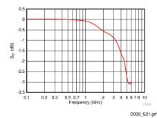
Figure 8-2. Insertion Loss Vs. Frequency
