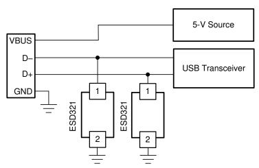
Figure 8-1. USB 2.0 ESD Schematic
