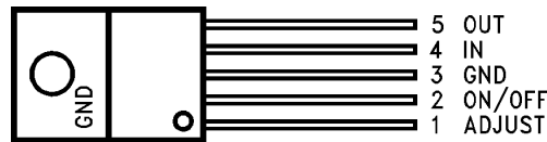
Figure 8. TO-220 5-Lead Power Package Front View
