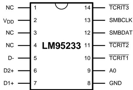
Figure 1. 14-Lead WSON - TOP VIEW
