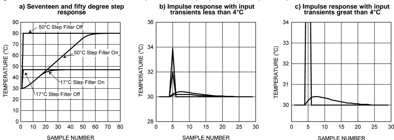
Figure 11. Filter Impulse and Step Response Curves
