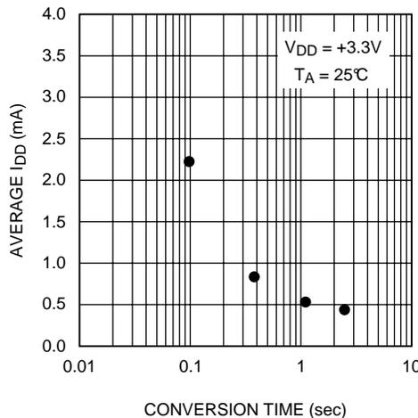
**Figure 10. Conversion Rate Effect on Power Supply Current**
