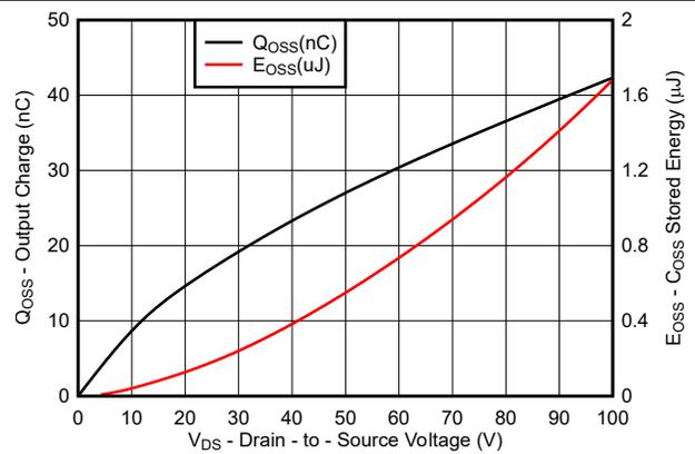
**Figure 5-12. LMG3100R044 Typical Output Charge and  $C_{OSS}$  Stored Energy**
