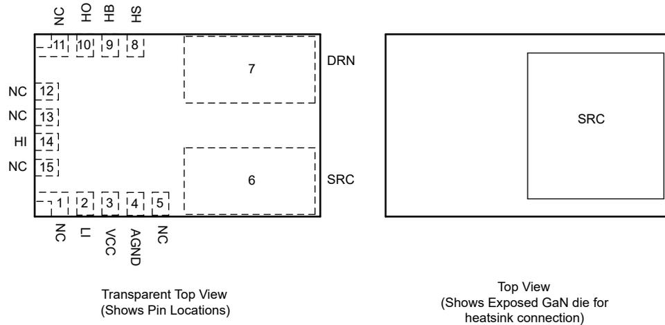
**Figure 4-1. VBE Package, 15-Pin VQFN (Top View)**
