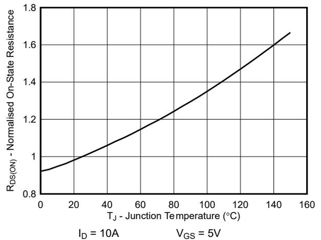
**Figure 5-14. LMG3100R044 Normalized On-State Resistance vs Junction Temperature**
