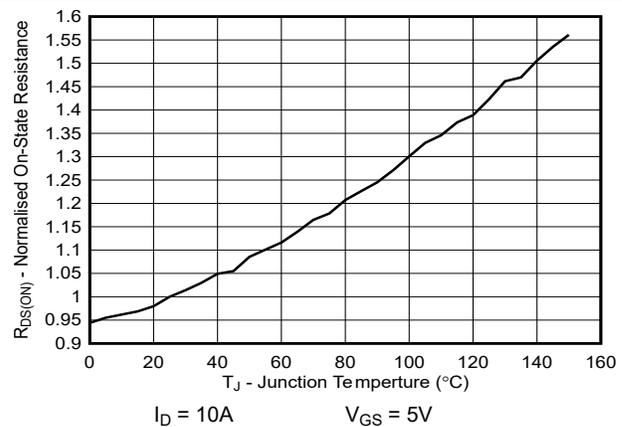
Figure 5-6. LMG3100R017 Normalized On-State Resistance vs Junction Temperature
