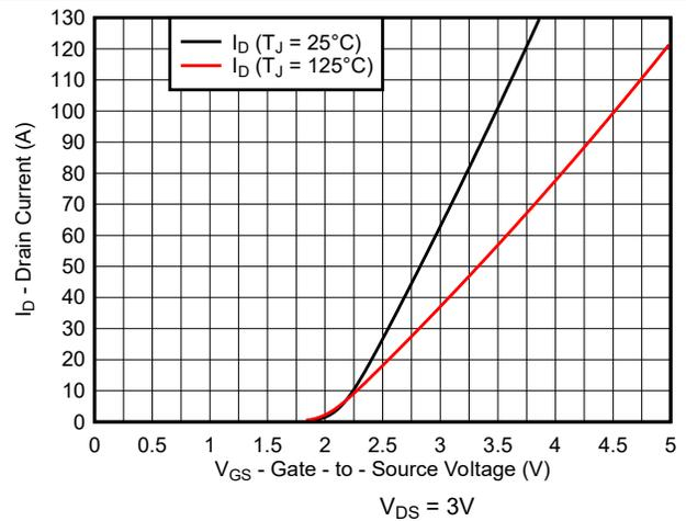
**Figure 5-10. LMG3100R044 Typical Transfer Characteristics**
