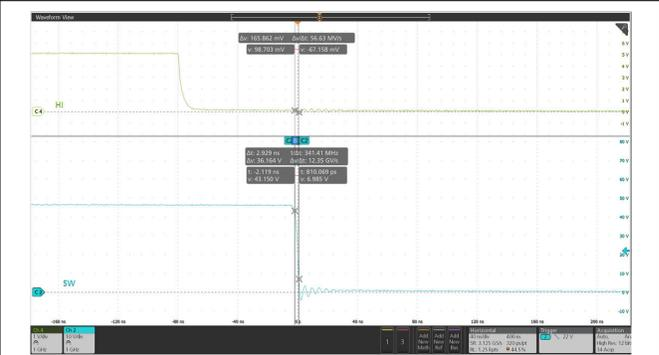
$I_{OUT} = 20\text{ A}$        $V_{IN} = 48\text{ V}$        $V_{OUT} = 24\text{ V}$
