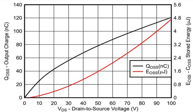
Figure 5-4. LMG3100R017 Typical Output Charge and  $C_{OSS}$  Stored Energy
