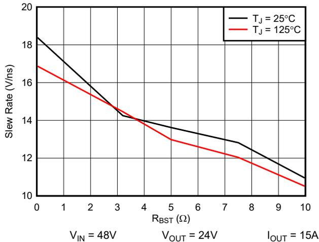
**Figure 5-15. LMG3100R044 Slew Rate Control for a Buck Converter Using R<sub>BST</sub>**
