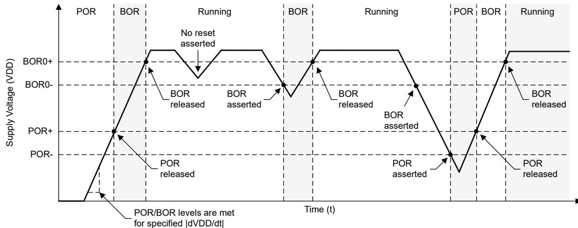
Figure 7-1. Power Cycle POR/BOR Conditions - VDD
