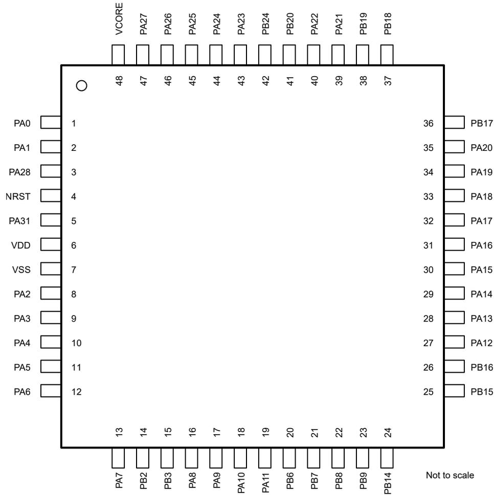
**Figure 6-5. 48-pin PT (0.5mm) (LQFP) Package Diagram**
