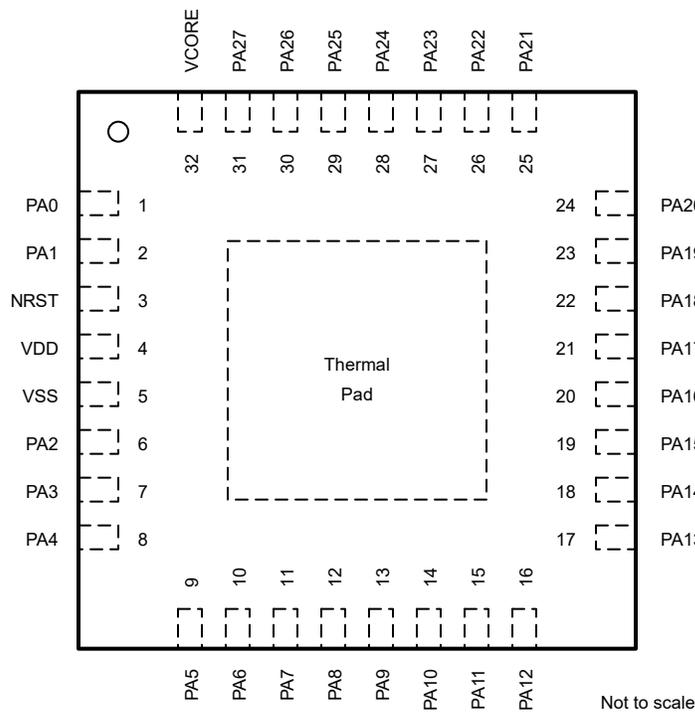
**Figure 6-8. 32-pin RHB (0.5mm) (VQFN) Package Diagram**
