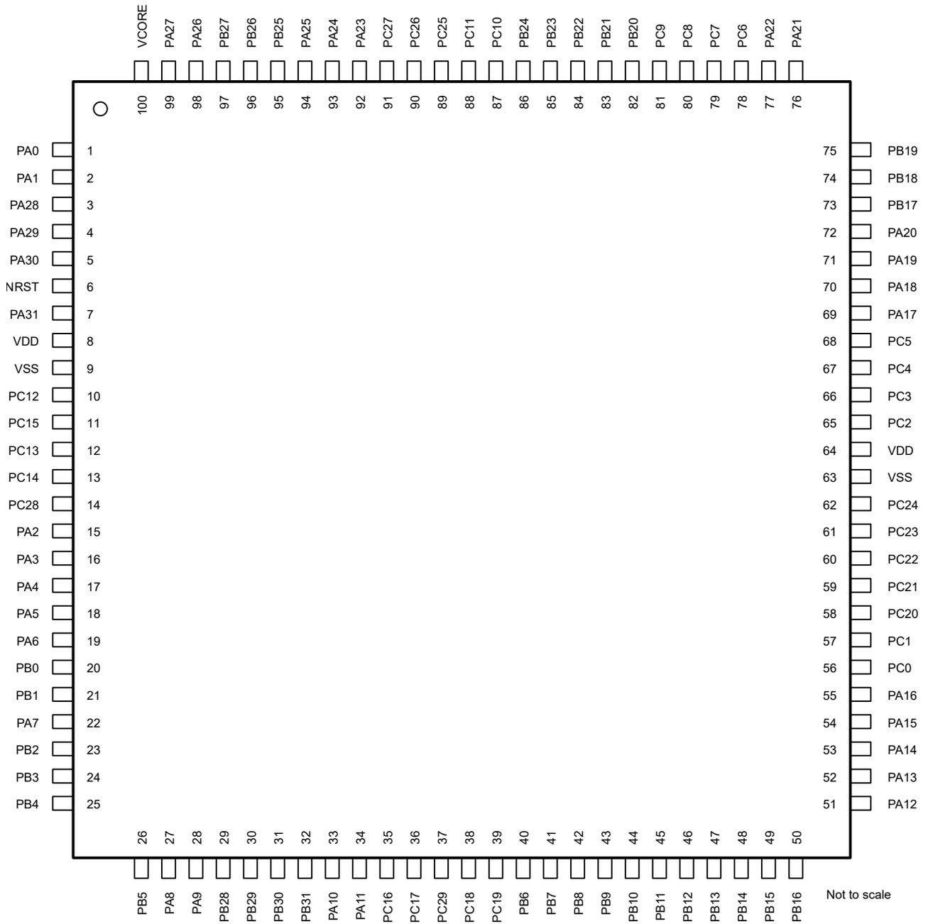
**Figure 6-2. 100-pin PZ (0.5mm) (LQFP) Package Diagram**
