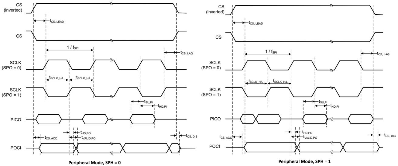
**Figure 7-5. SPI timing diagram - Peripheral Mode**
