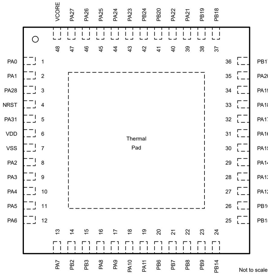
**Figure 6-6. 48-pin RGZ (0.5mm) (VQFN) Package Diagram**
