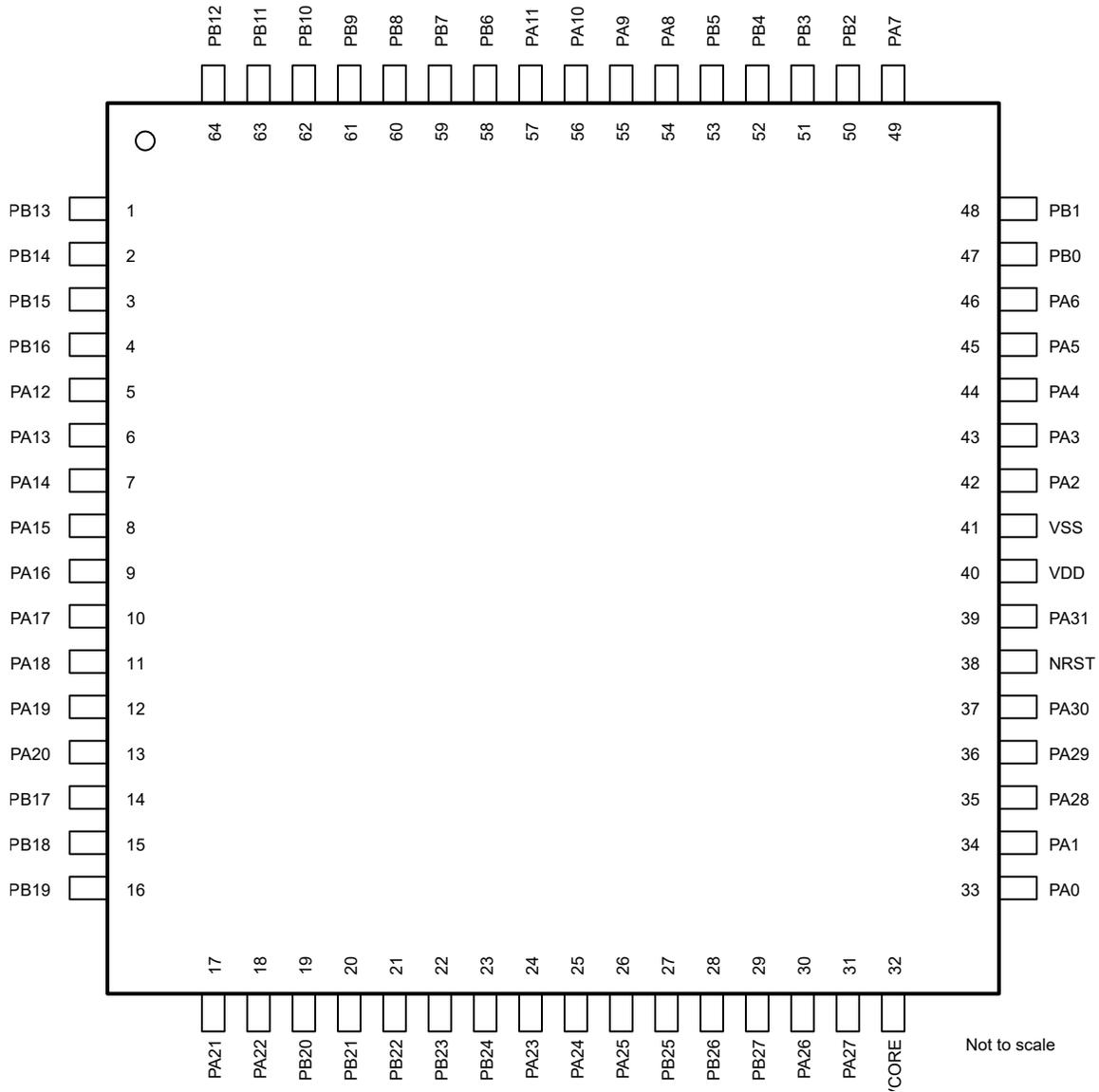
**Figure 6-4. 64-pin PM (0.5mm) (LQFP) Package Diagram**
