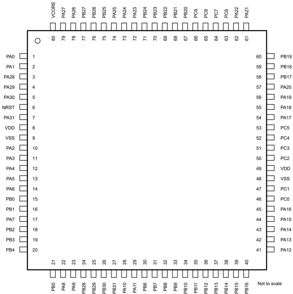
**Figure 6-3. 80-pin PN (0.5mm) (LQFP) Package Diagram**
