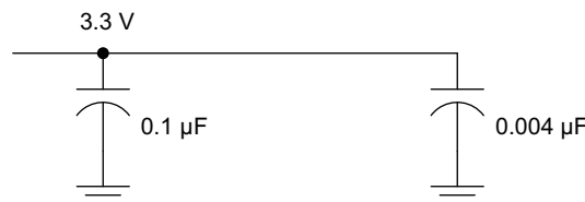
Figure 9-2. Recommended M-LVDS Bypass Capacitor Layout
