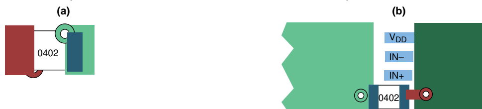
Figure 28. Typical Decoupling Capacitor Layouts
