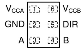
**Figure 5-4. DRY Package 6-Pin SON Transparent Top View**
