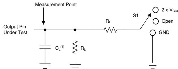
A.  $C_L$  includes probe and jig capacitance.
