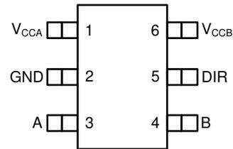
**Figure 5-2. DCK Package 6-Pin SC70 Top View**
