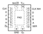
Figure 5-2. RGY or BQB Package, 16-Pin VQFN or WQFN (Top View)
