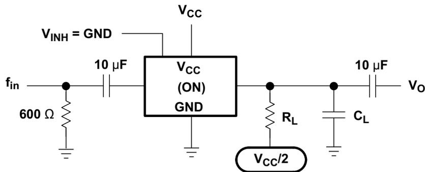
Figure 6-9. Sine-Wave Distortion
