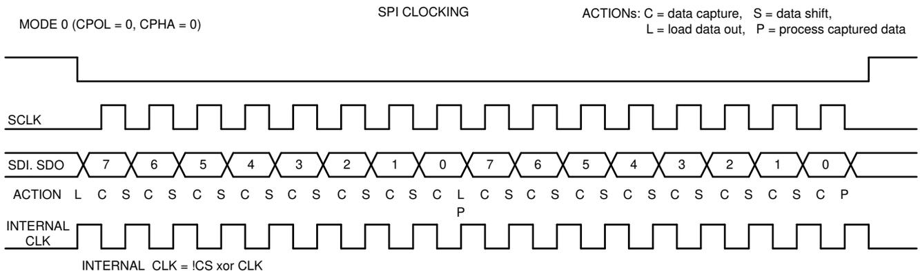
Figure 8-17. SPI Clocking
