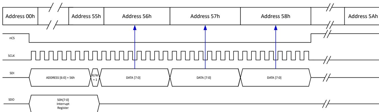
Figure 8-19. 32-bit SPI Burst Write
