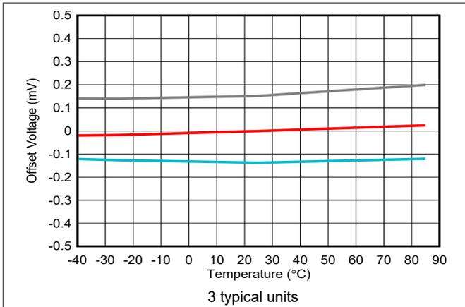
Figure 5-25. Input Offset Voltage vs Ambient Temperature
