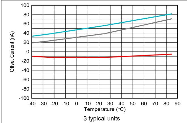
Figure 5-27. Input Offset Current vs Ambient Temperature
