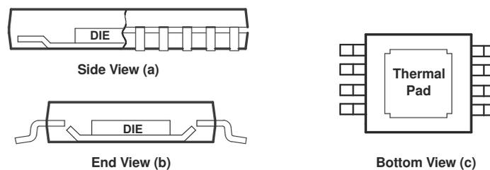
Note: The thermal pad is electrically isolated from all pins in the package.
