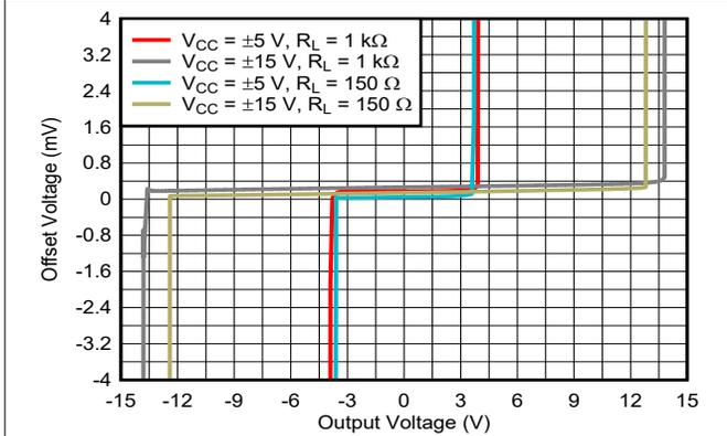
Figure 5-29. Offset Voltage vs Output Voltage
