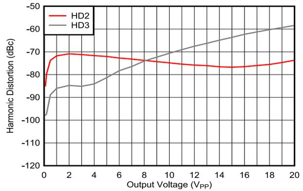
$V_{CC} = \pm 15\text{V}$ , gain =  $+5\text{V/V}$ ,  $R_L = 150\Omega$ ,  $f = 1\text{MHz}$
