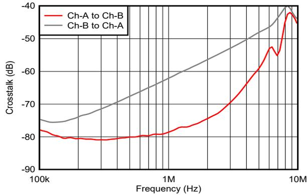
$V_{CC} = \pm 15\text{V}$ , gain =  $+2\text{V/V}$
