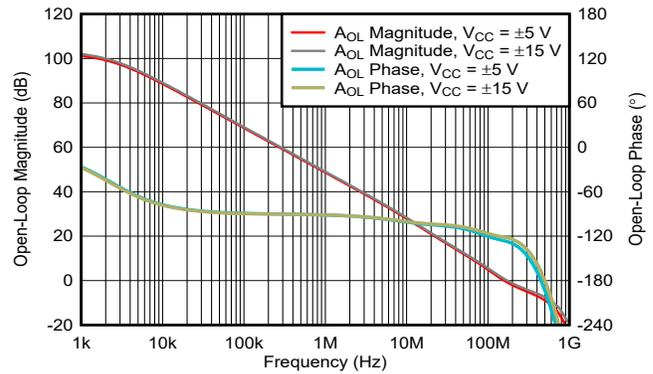
Figure 5-10. Open-Loop Gain and Phase Response
