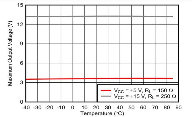
Figure 5-30. Maximum Output Voltage Swing vs Ambient Temperature
