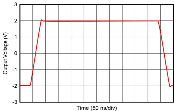
$V_{CC} = \pm 5\text{V}$ , gain =  $-1\text{V/V}$ ,  $R_F = 430\Omega$
