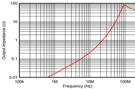
Figure 5-9. Closed-Loop Output Impedance
