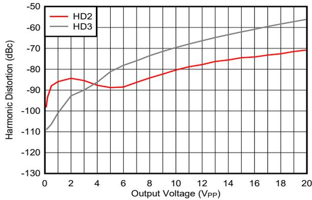
$V_{CC} = \pm 15\text{V}$ , gain =  $+5\text{V/V}$ ,  $R_L = 1\text{k}\Omega$ ,  $f = 1\text{MHz}$
