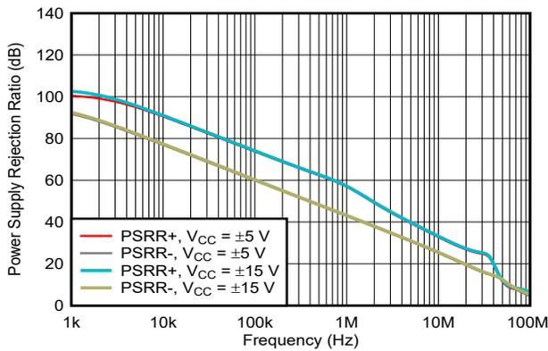
Figure 5-11. Power-Supply Rejection Ratio vs Frequency
