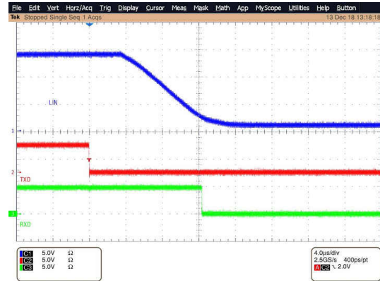
Figure 9-12. Recessive to Dominant Propagation Delay
