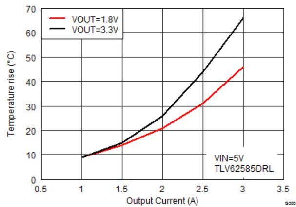
Figure 22. Temperature Rise of DRL Package on EVM
