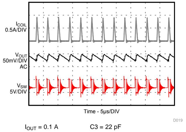
Figure 14. PSM Operation with a Feedforward Capacitor
