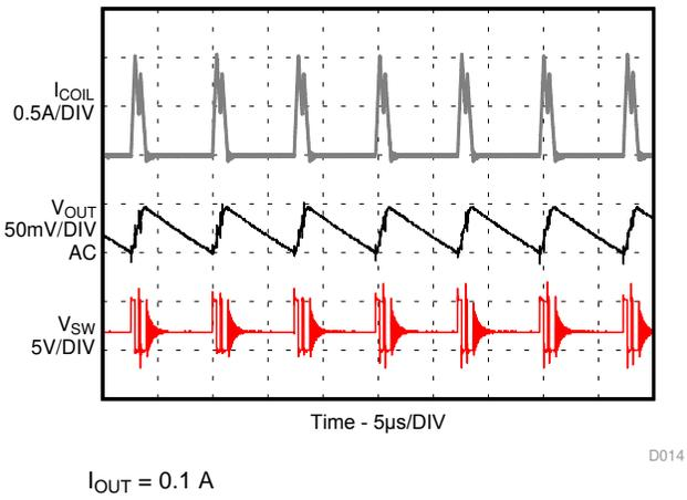
Figure 13. PSM Operation
