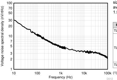
**Noise Spectral Density vs Frequency**
