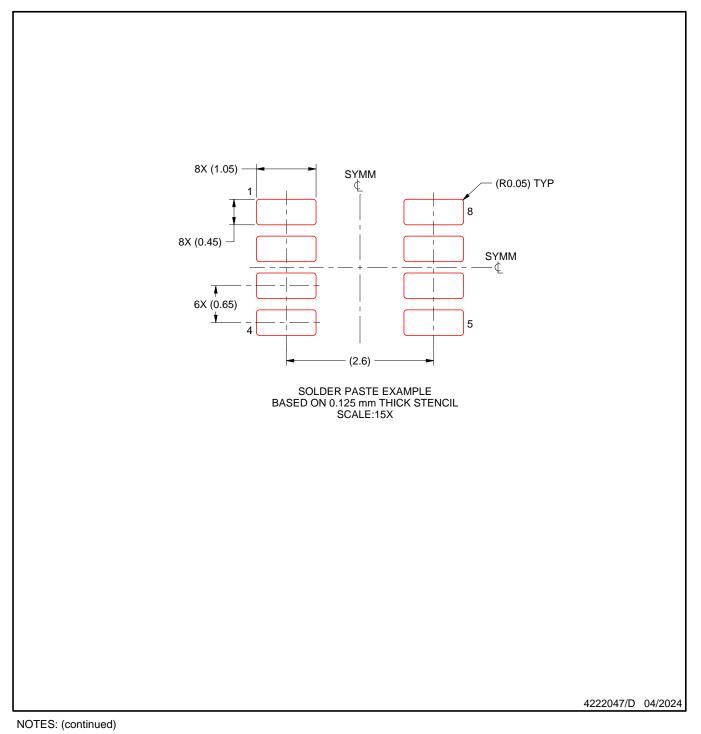
6. Laser cutting apertures with trapezoidal walls and rounded corners may offer better paste release. IPC-7525 may have alternate design recommendations.
