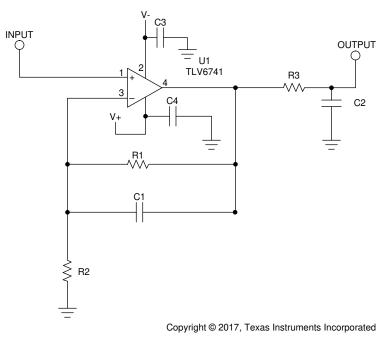
Figure 11-2. Schematic Used for Layout Example
