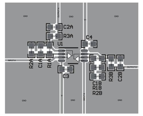
Figure 11-3. Example Layout for VSSOP-8 (DGK) Package
