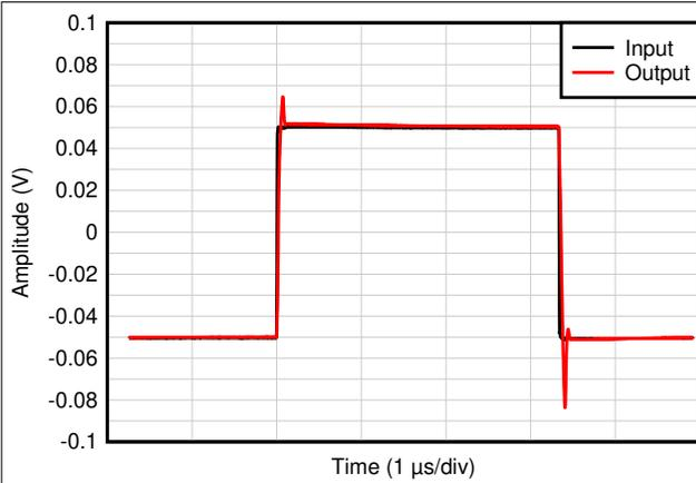
$C_L = 20\text{ pF}$ , Gain = 1,  $V_{IN} = 100\text{-mVpp}$ ,  $R_L = 1\text{ k}\Omega$
