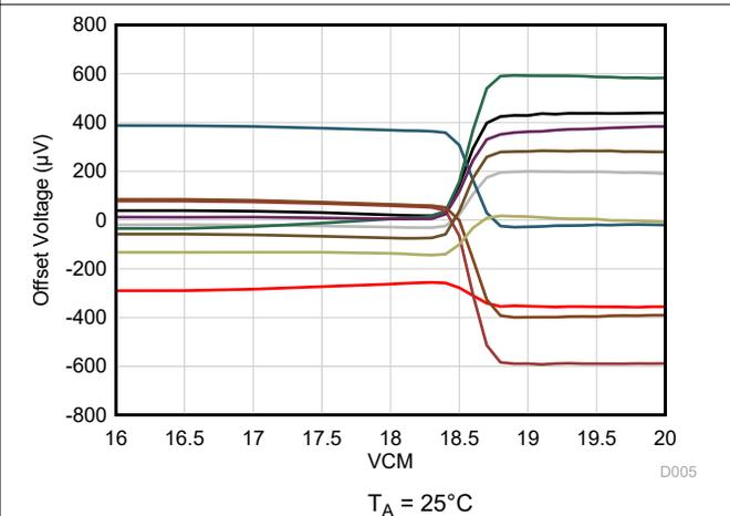
**Figure 5-6. Offset Voltage vs Common-Mode Voltage (Transition Region)**
