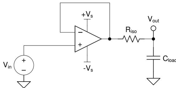
**Figure 6-7. Extending Capacitive Load Drive With the TLV9351-Q1**
