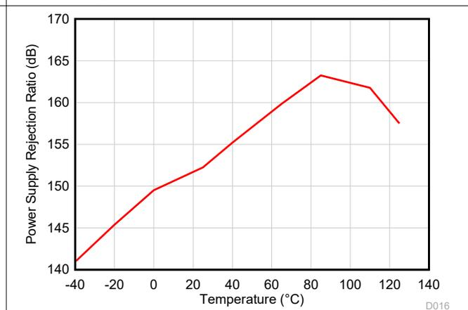
Figure 5-18. PSRR vs Temperature (dB)
