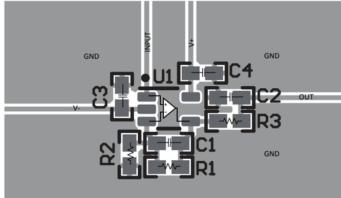
Figure 7-5. Example Layout for SC70 (DCK) Package
