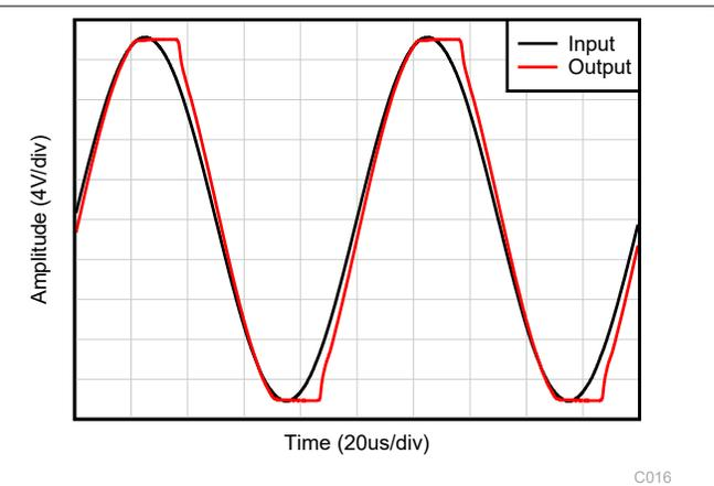
$V_{IN} = \pm 20\text{ V}$ ;  $V_S = V_{OUT} = \pm 17\text{ V}$
