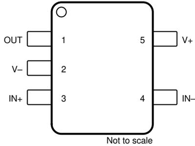
**Figure 4-1. TLV9351-Q1 DBV Package,
