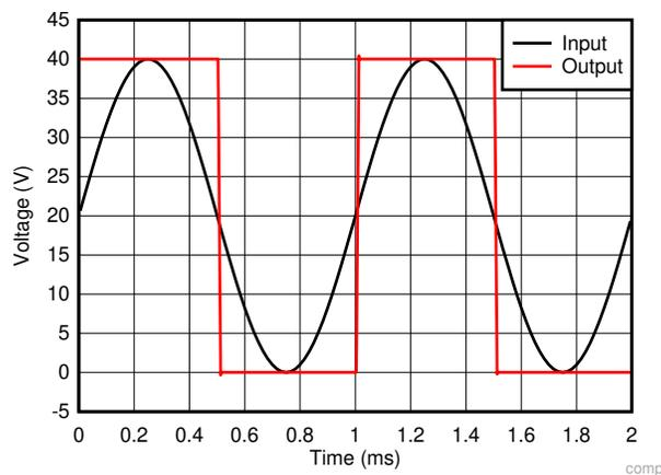
**Figure 7-2. Comparator Output Response to Input Voltage**
