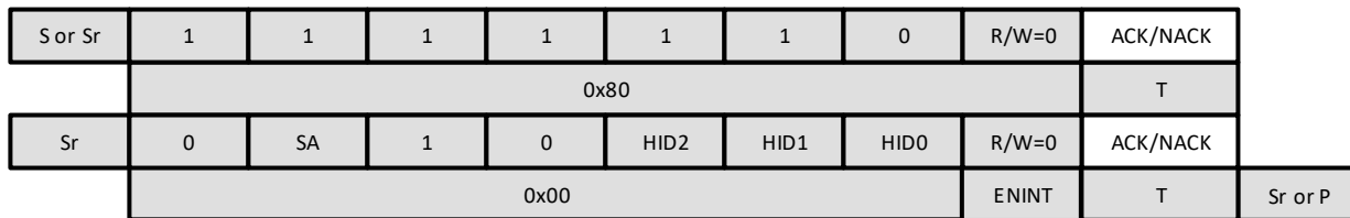
Figure 7-26. ENEC CCC Direct
