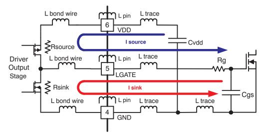
Figure 28. MOSFET Drive Paths and Main Circuit Parasitics
