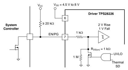
Figure 20. Enable/Power Good Circuit
