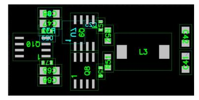
Figure 41. Component Placement Based on Schematic in Figure 25
