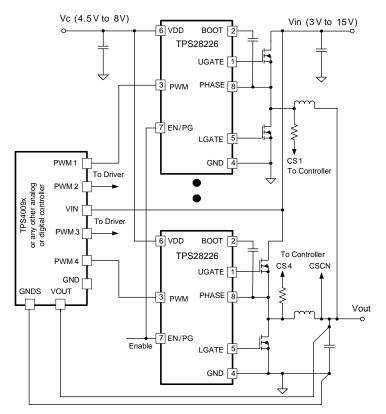
Figure 38. Multi-Phase Synchronous Buck Converter
