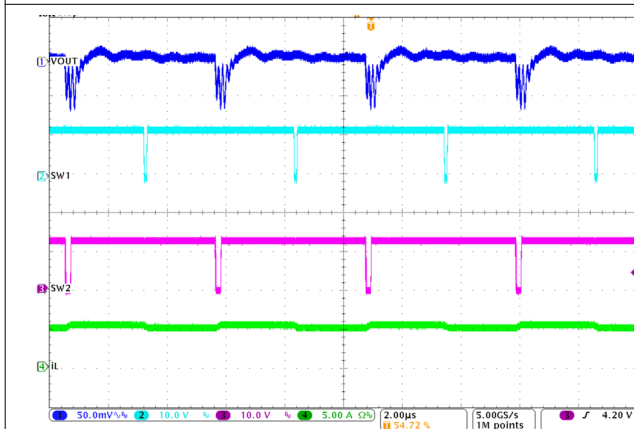
Figure 8-4. Switching Waveforms in V_{IN} = 12\text{ V} , V_{OUT} = 12\text{ V} , I_O = 5\text{ A} , FPWM
