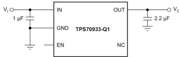
Figure 7-1. 3.3-V, Low-I<sub>Q</sub> Rail
