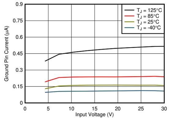
Figure 5-22. 3.3-V Shutdown Current vs  $V_{IN}$  and Temperature
