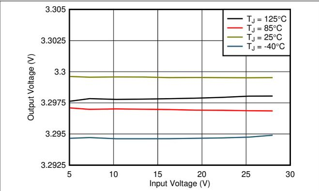
**Figure 5-2. 3.3-V Line Regulation vs  $V_{IN}$  and Temperature**
