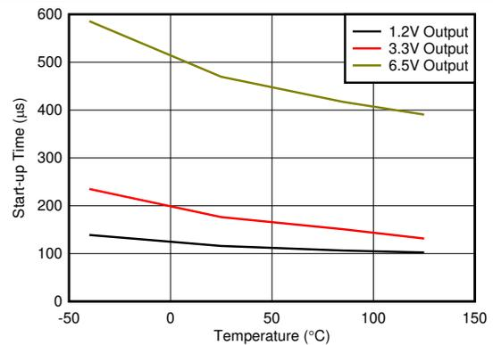
Figure 5-24. Start-Up Time vs Temperature
