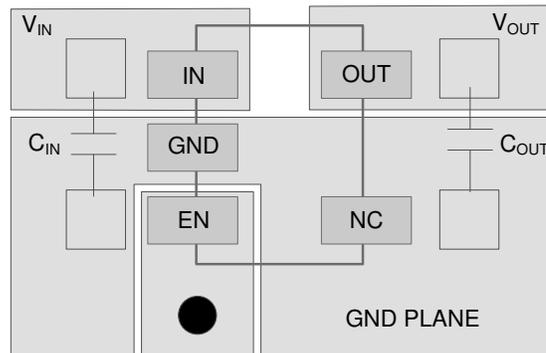
● Represents via used for application-specific connections.
