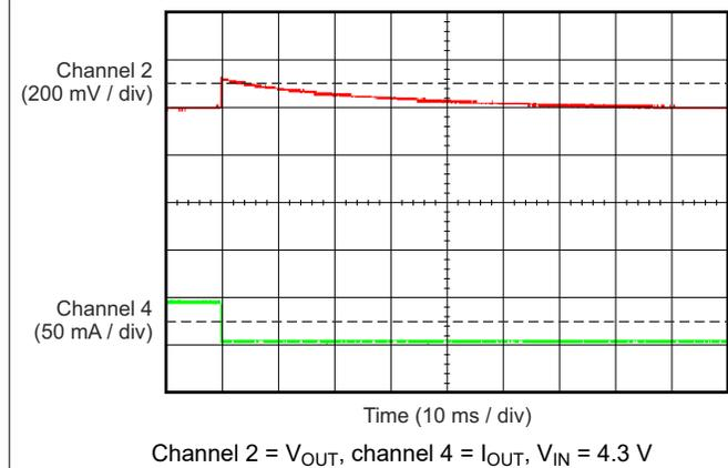
**Figure 5-33. TPS70933-Q1 Load Transient (50 mA to 0 mA)**
