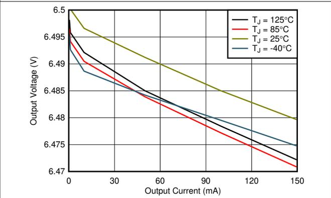
**Figure 5-6. 6.5-V Load Regulation vs  $I_{OUT}$  and Temperature**
