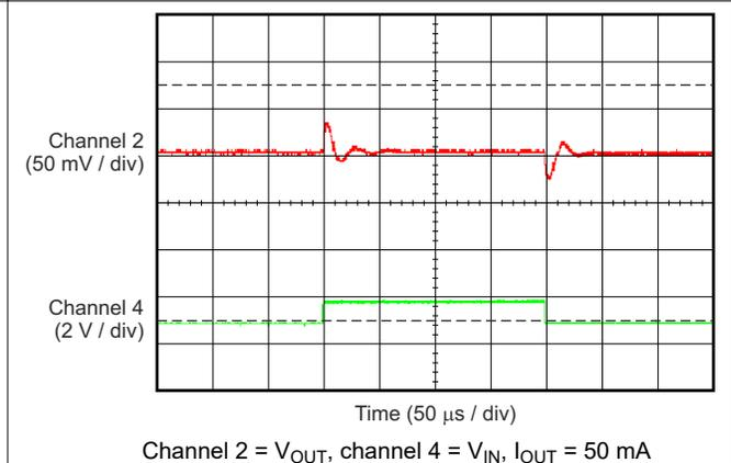
**Figure 5-36. TPS70912-Q1 Line Transient (2.7 V to 3.7 V)**
