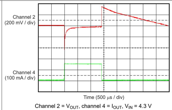
**Figure 5-32. TPS70933-Q1 Load Transient (1 mA to 150 mA)**
