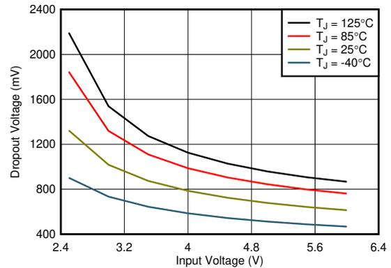
Figure 5-8. 6.5-V Dropout Voltage vs  $V_{IN}$  and Temperature
