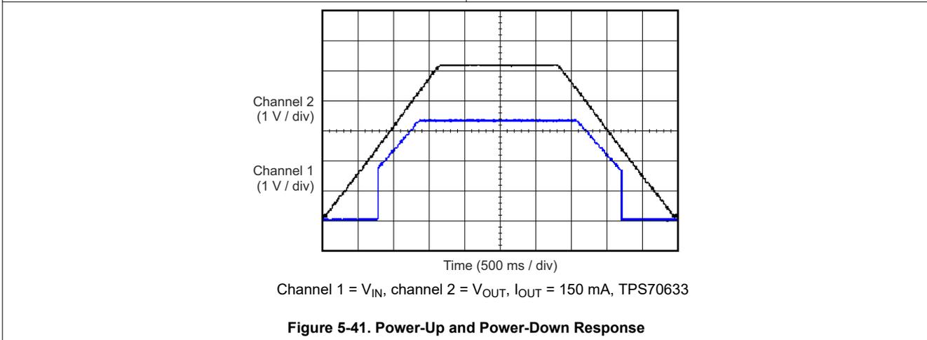
**Figure 5-41. Power-Up and Power-Down Response**
