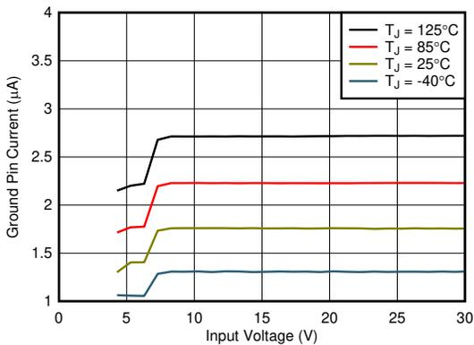
Figure 5-17. 3.3-V Ground Current vs  $V_{IN}$  and Temperature with EN Floating
