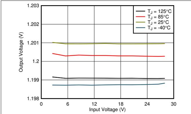
**Figure 5-1. 1.2-V Line Regulation vs  $V_{IN}$  and Temperature**
