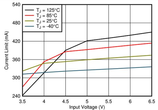
Figure 5-11. 1.2-V Current Limit vs  $V_{IN}$  and Temperature
