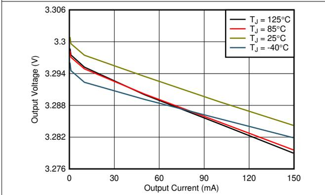
**Figure 5-5. 3.3-V Load Regulation vs  $I_{OUT}$  and Temperature**
