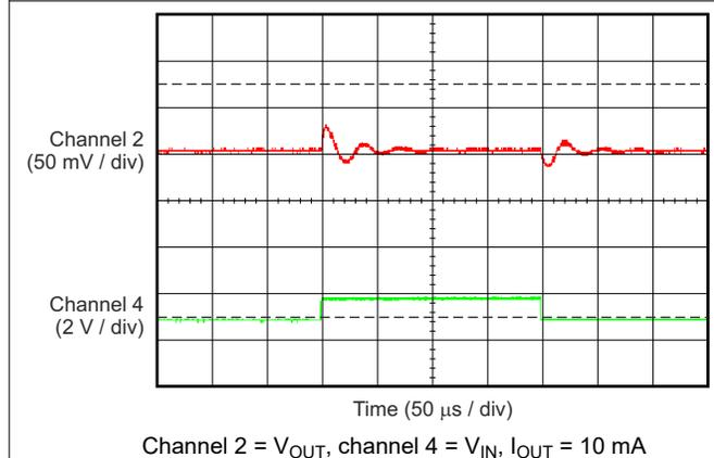
**Figure 5-35. TPS70912-Q1 Line Transient (2.7 V to 3.7 V)**
