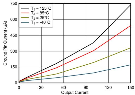
Figure 5-18. 1.2-V Ground Pin Current vs  $I_{OUT}$  and Temperature
