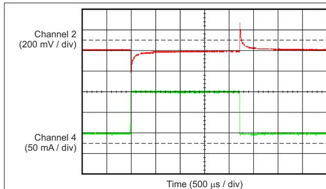
Channel 2 = V<sub>OUT</sub>, channel 4 = I<sub>OUT</sub>, V<sub>IN</sub> = 4.3 V
