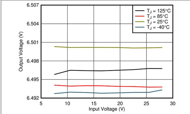
**Figure 5-3. 6.5-V Line Regulation vs  $V_{IN}$  and Temperature**
