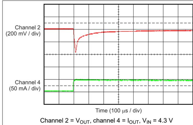
**Figure 5-31. TPS70933-Q1 Load Transient (0 mA to 50 mA)**
