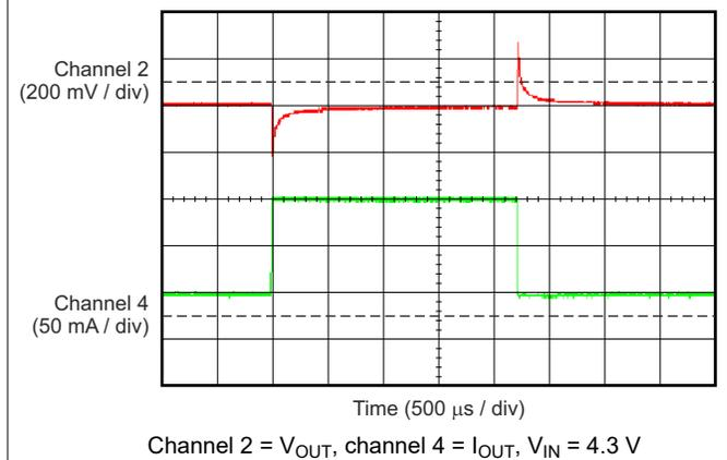
**Figure 5-34. TPS70933-Q1 Load Transient (50 mA to 150 mA)**
