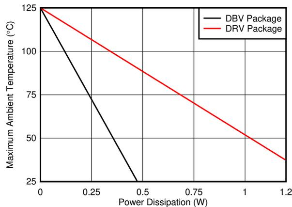
**Figure 7-4. Maximum Ambient Temperature vs Device Power Dissipation**
