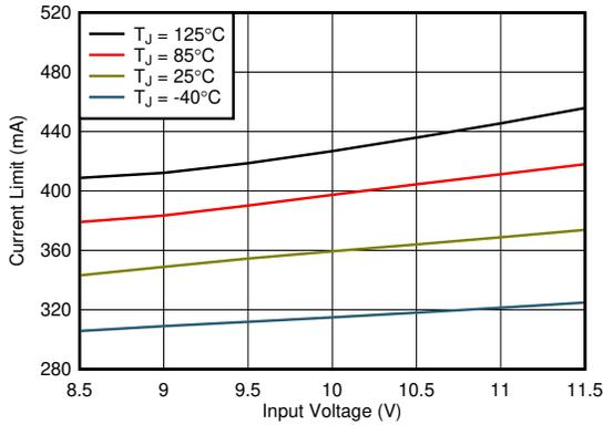
Figure 5-13. 6.5-V Current Limit vs  $V_{IN}$  and Temperature
