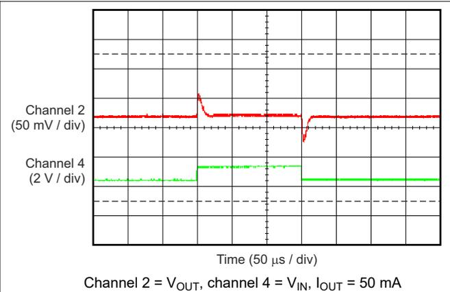
**Figure 5-38. TPS70933-Q1 Line Transient (4.3 V to 5.3 V)**
