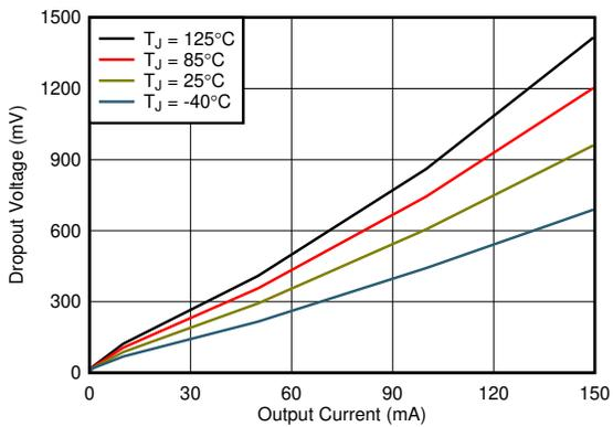
Figure 5-9. 3.3-V Dropout Voltage vs  $I_{OUT}$  and Temperature
