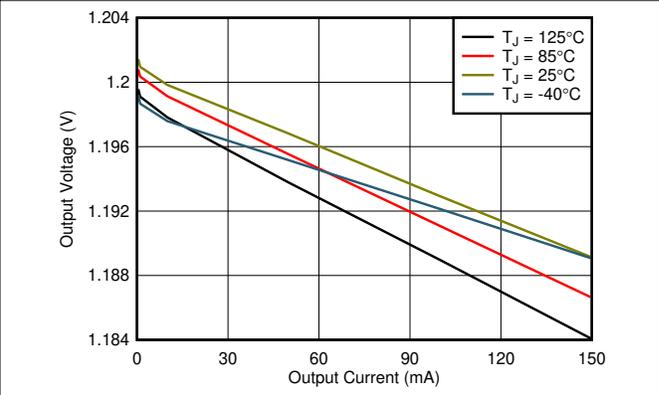
**Figure 5-4. 1.2-V Load Regulation vs  $I_{OUT}$  and Temperature**
