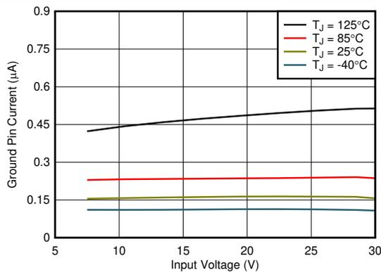
Figure 5-23. 6.5-V Shutdown Current vs  $V_{IN}$  and Temperature
