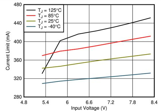
Figure 5-12. 3.3-V Current Limit vs  $V_{IN}$  and Temperature
