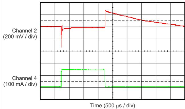
Channel 2 =  $V_{OUT}$ , channel 4 =  $I_{OUT}$ ,  $V_{IN} = 2.7\text{ V}$
