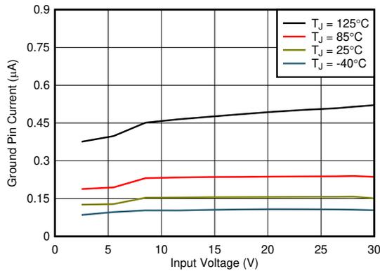
Figure 5-21. 1.2-V Shutdown Current vs  $V_{IN}$  and Temperature
