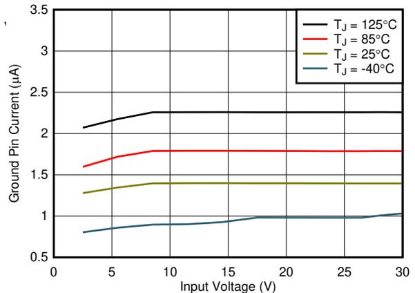
**GND Current vs V<sub>IN</sub> and Temperature**
