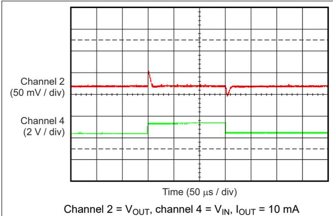
**Figure 5-37. TPS70933-Q1 Line Transient (4.3 V to 5.3 V)**
