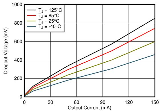
Figure 5-10. Dropout Voltage vs  $I_{OUT}$  and Temperature
