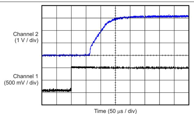
Channel 1 = EN, channel 2 = V<sub>OUT</sub>, V<sub>IN</sub> = 4.3 V, C<sub>OUT</sub> = 2.2 µF, TPS70933-Q1
