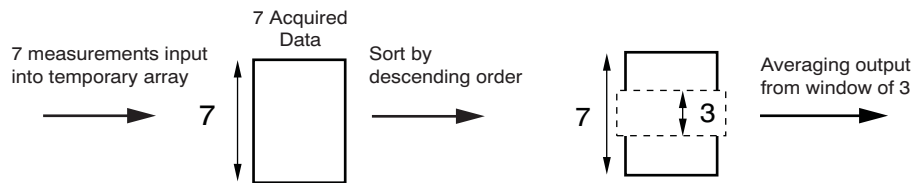
Figure 28. MAV Filter Operation (Patent Pending)
