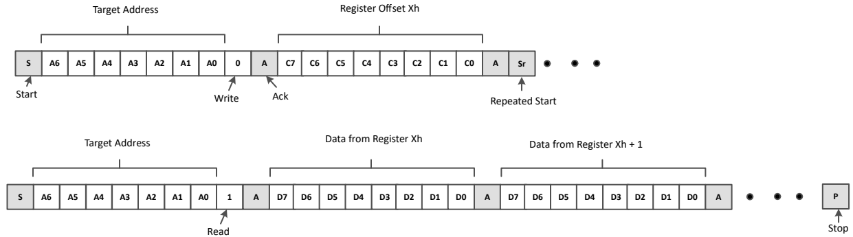
Figure 6-4. I2C Read with Repeated Start
