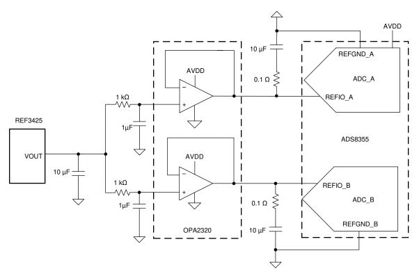
Figure 45. Reference Drive Circuit
