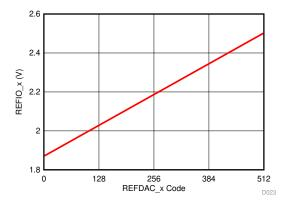
Figure 25. REFDAC Transfer Function
