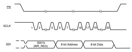
Figure 32. Register Write Operation
