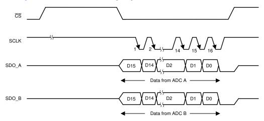
Figure 29. Dual-SDO Mode Timing Diagram
