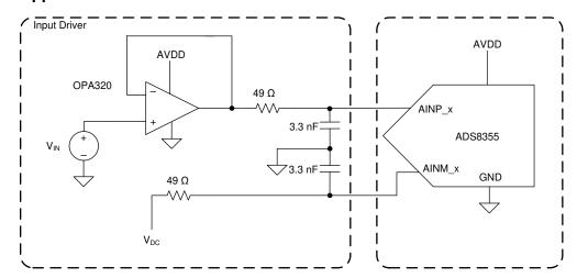
NOTE: Only one ADC channel is shown in this diagram. Replicate the same circuit for the other ADC channel.
