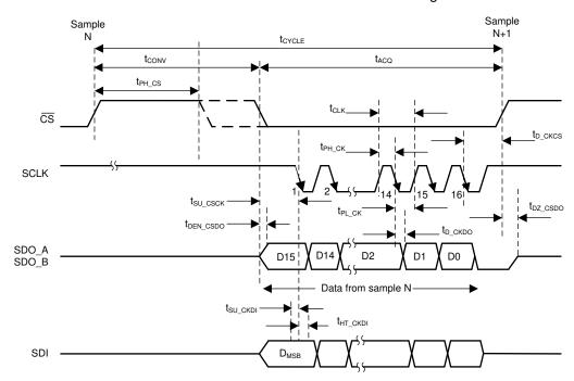
Figure 1. Serial interface Timing Diagram
