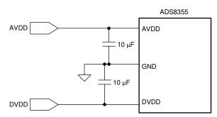
Figure 47. Power-Supply Decoupling
