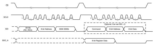
Figure 31. Register Read Operation
