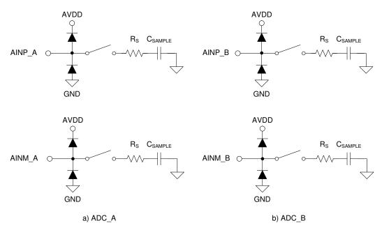
Figure 26. Equivalent Circuit for the Analog Input Pins
