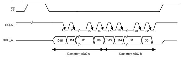
Figure 30. Single-SDO Mode Timing Diagram
