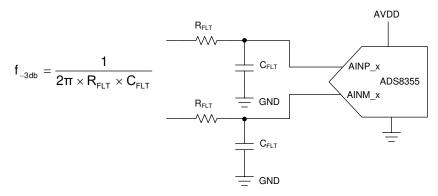
Figure 43. Charge Kickback Filter
