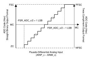
Figure 28. Ideal Transfer Characteristics for a Pseudo-Differential Analog Input
