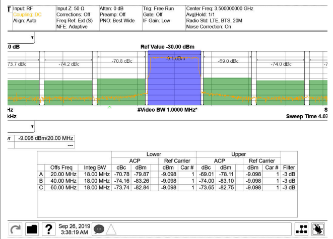
3.5 GHz Matching, single carrier 20-MHz BW TM1.1 LTE Figure 5-449. TX 20-MHz LTE Output Spectrum at 3.5 GHz (Band 42)
