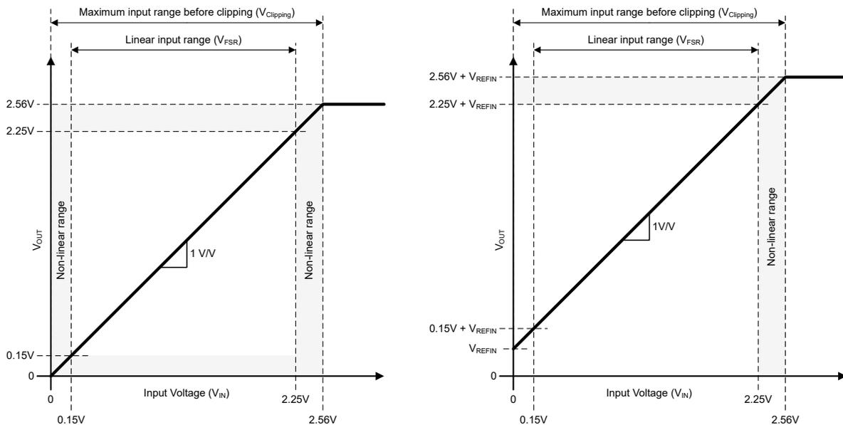
**Figure 7-2. Input-to-Output Transfer Curve of the AMC0x11S-Q1**
