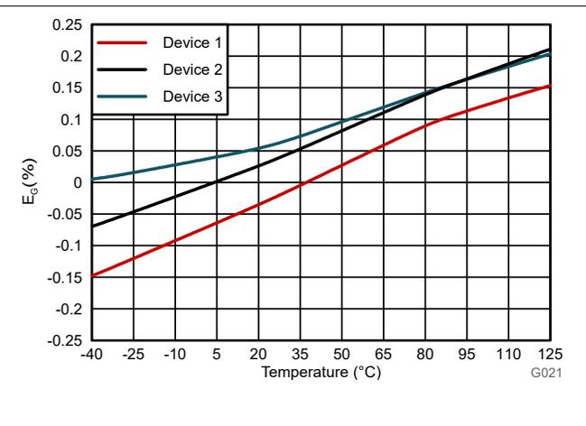
Figure 6-9. Gain Error vs Temperature
