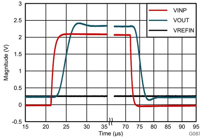
**Figure 8-4. Step Response of the AMC0x11S-Q1**
