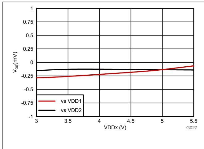
Figure 6-6. Input Offset Voltage vs Supply Voltage
