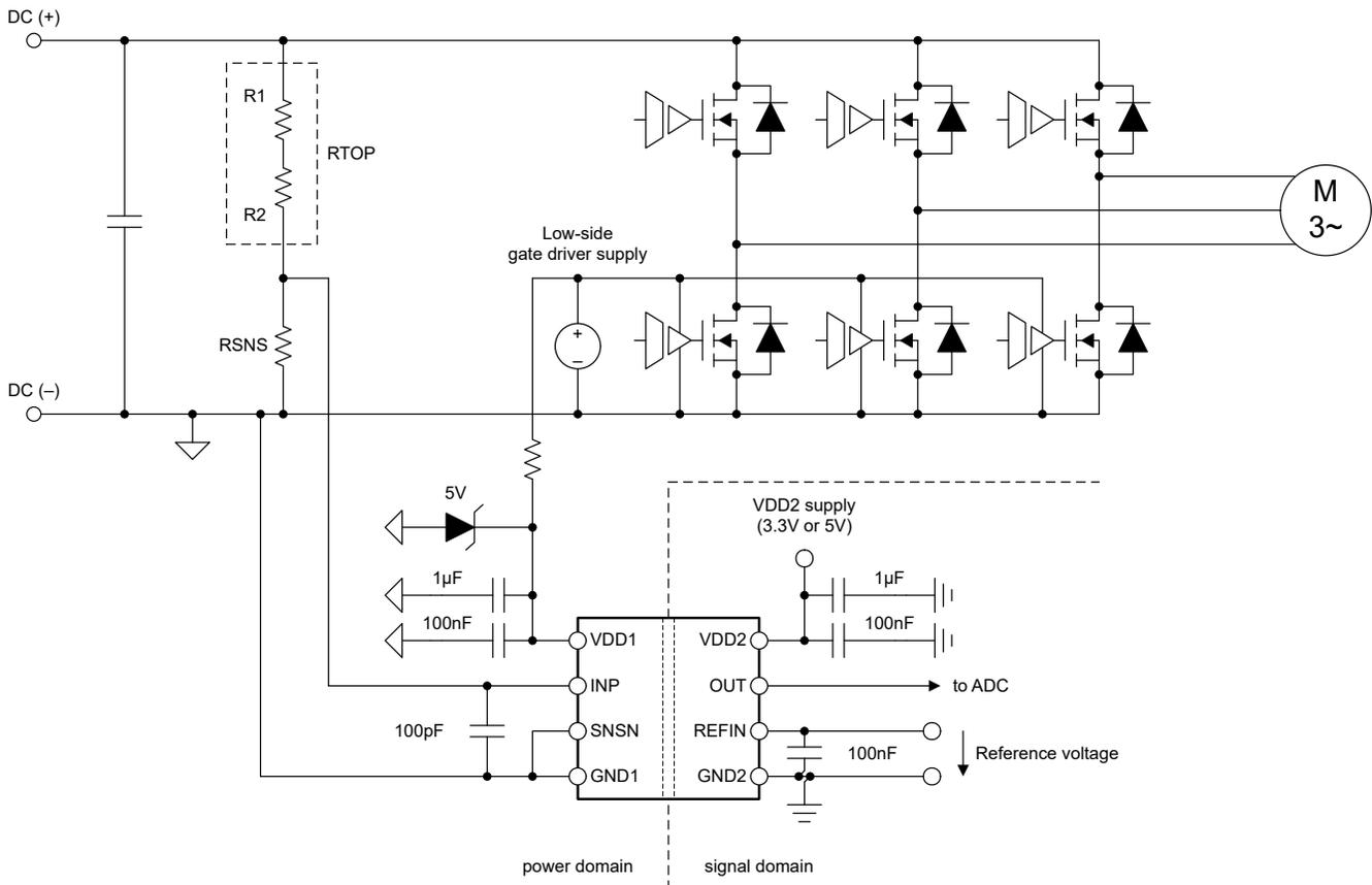
Figure 8-1. Using the AMC0x11S-Q1 in a Typical Application
