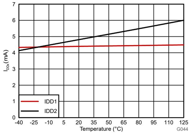
Figure 6-14. Supply Current vs Temperature
