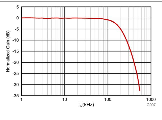
Figure 6-11. Normalized Gain vs Input Frequency
