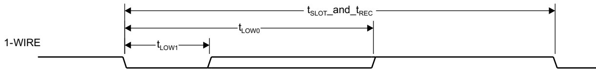
Figure 5-109. 1-Wire Write Bit Timing (Command/Address or Data)
