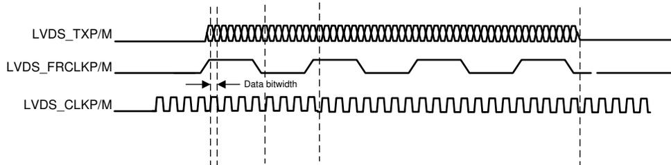
Figure 7-17. LVDS Interface Lane Configuration And Relative Timings
