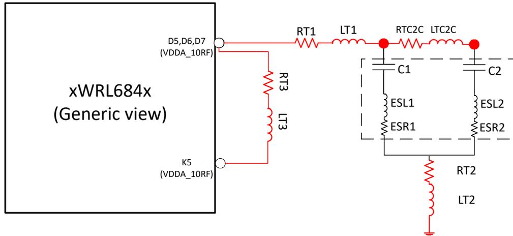
**Figure 7-5. Parasitic offered by different portion of the output path for two capacitors**
