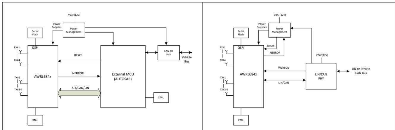
**Figure 7-1. System Topologies (Left : Topology 1, Right : Topology 2)**
