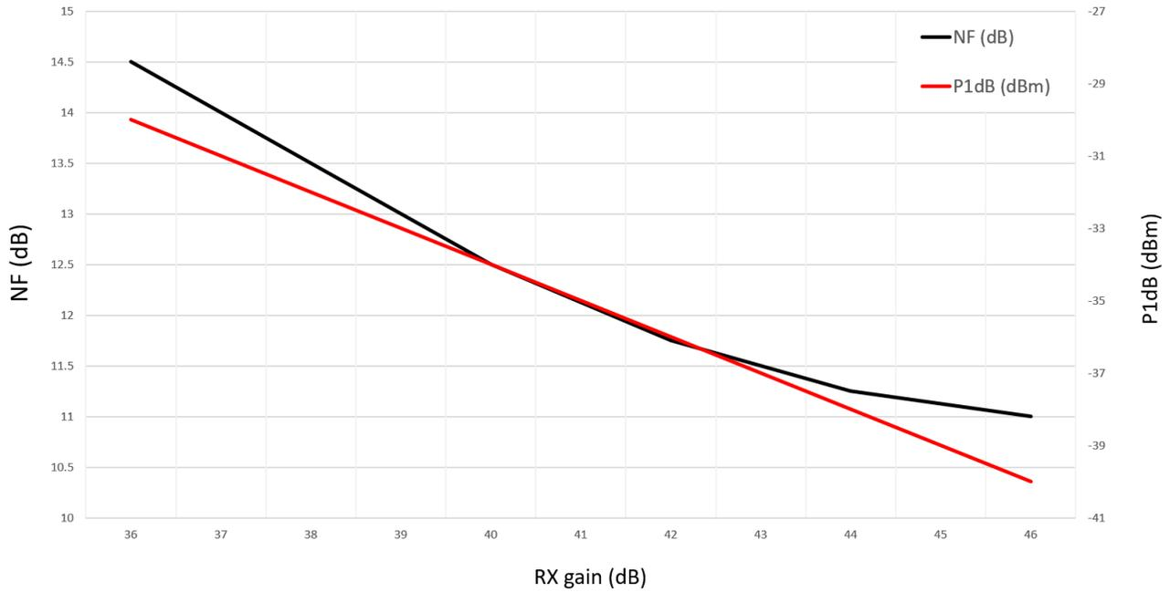
**Figure 7-8. Noise Figure, In-band P1dB vs Receiver Gain**
