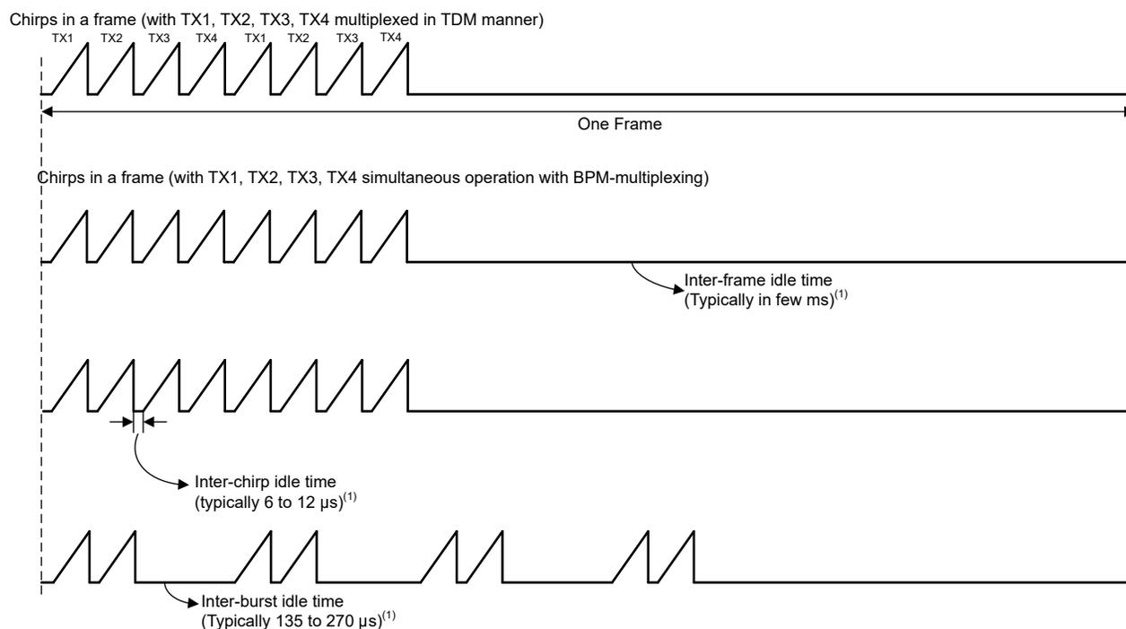
**Figure 7-9. Chip Profile Supported by Timing Engine**
