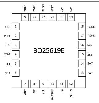
Figure 6-2. BQ25619E RTW Package 24-Pin WQFN Top View
