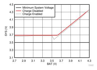
Figure 8-1. System Voltage vs Battery Voltage
