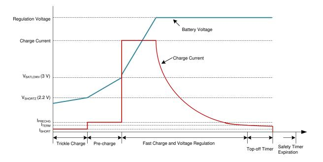
Figure 8-2. Battery Charging Profile
