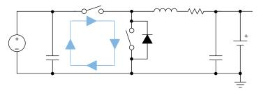
Figure 11-1. High Frequency Current Path
