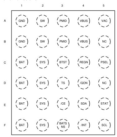
Figure 6-1. BQ25618E YFF Package 30-Pin WCSP Top View
