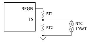
Figure 8-4. TS Pin Resistor Network
