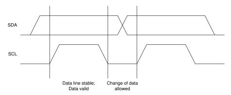
Figure 8-6. Bit Transfer on the I<sup>2</sup>C Bus
