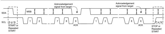
Figure 7-9. Data Transfer on the I<sup>2</sup>C Bus
