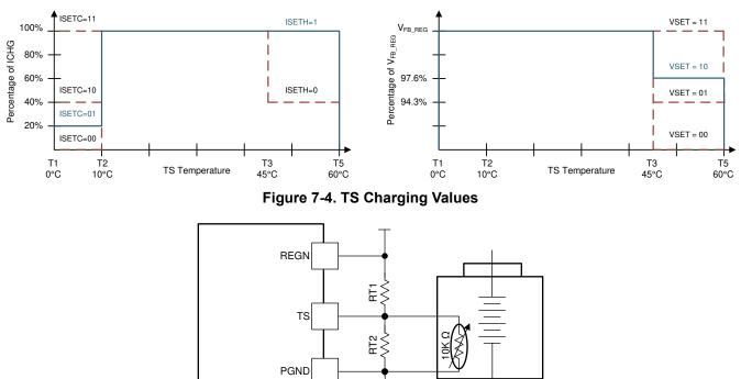
Assuming a 103AT NTC thermistor on the battery pack as shown above, the value of RT1 and RT2 can be determined by:
