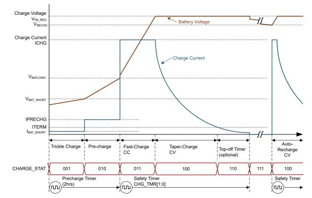
Figure 7-3. Typical Li-Ion Battery Charging Profile
