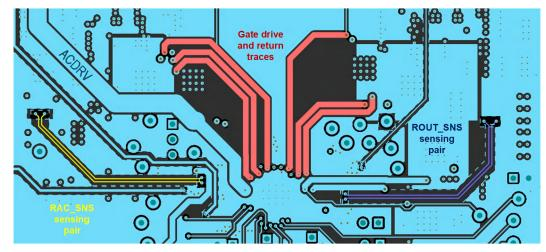
Figure 10-2. PCB Layout Gate Drive and Current Sensing Signal Layer Routing
