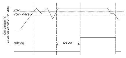
Figure 7-2. Timing for Overvoltage Sensing for OUT
