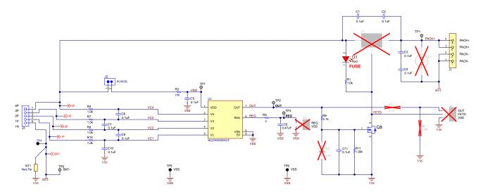
Figure 8-2. BQ2969 4-Series Cell Schematic Diagram - Protector and Fuse Blow Circuitry
