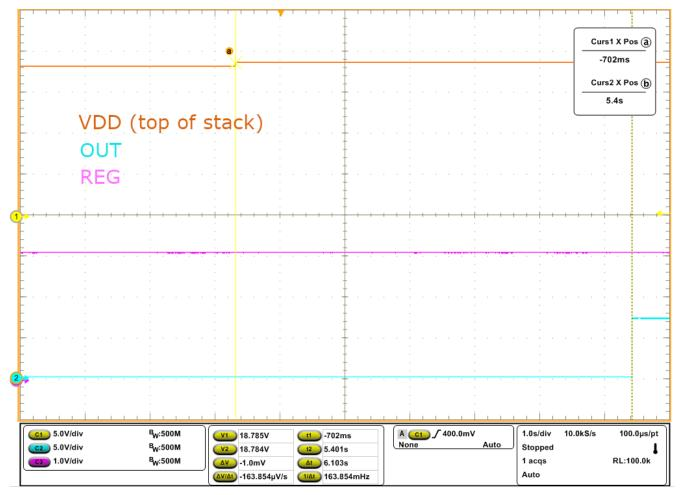
Figure 8-4. Overvoltage Protection Triggering
