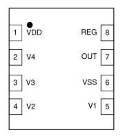
Figure 5-1. 2-Series to 4-Series BQ2969 (Top View)
